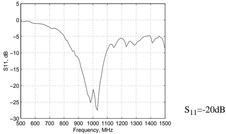
**Fig. 10.23** S11 of LNA with Bond-wire Inductors as Gate Inductors
