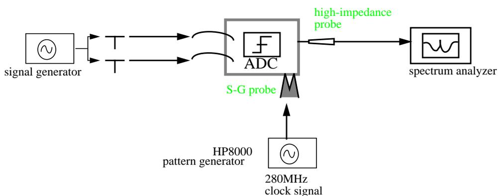
**Fig. 10.17** Setup of ADC Testing
