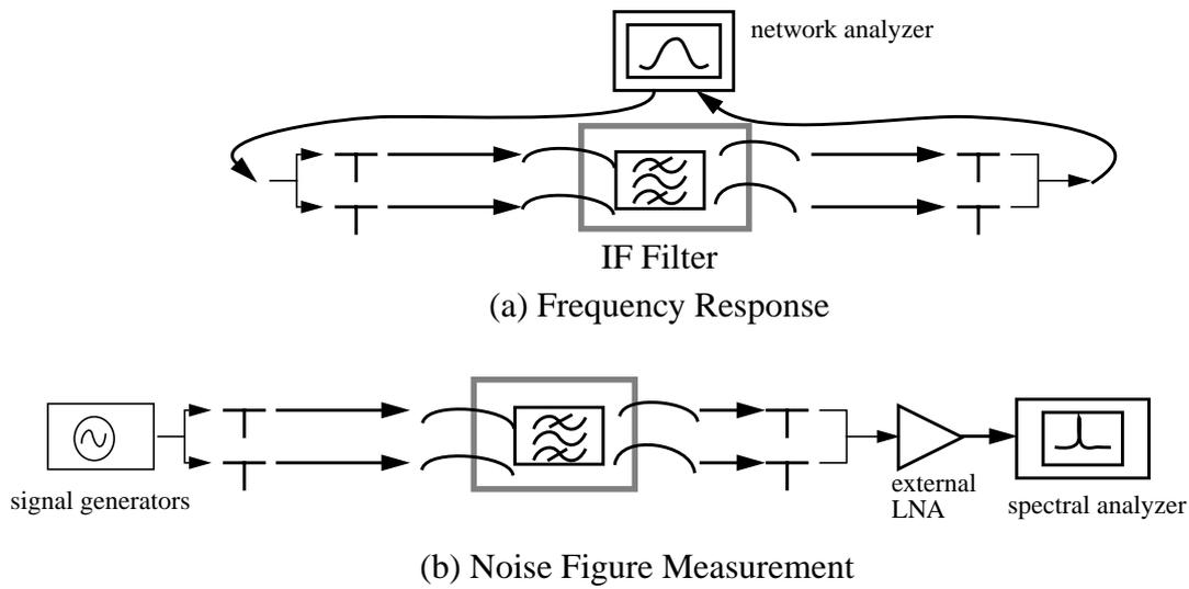
**Fig. 10.15** Setup of IF Filter Testing
