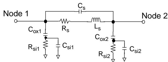
**Fig. 4.1** A complete inductor model
