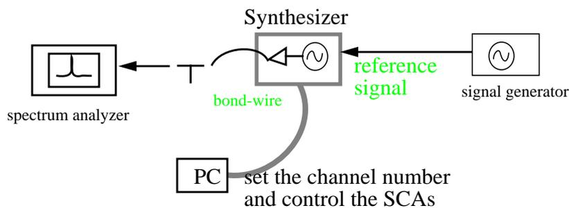
**Fig. 10.13** Setup of Synthesizer Testing
