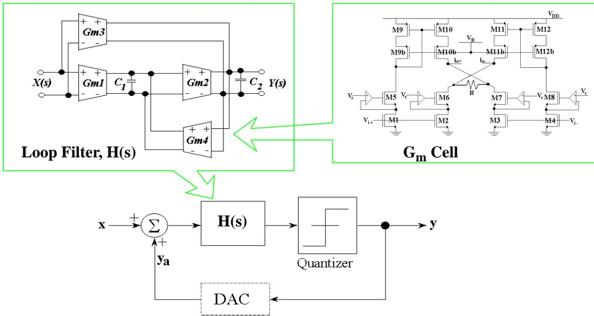
Fig. 8.5 Block diagram of the bandpass sigma-delta analog-to-digital converter
