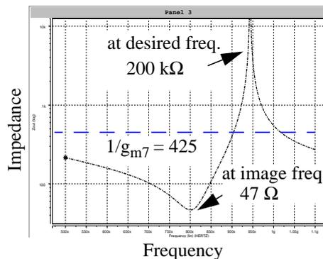
**Fig. 5.10** Input Impedance of the Notch Filter
