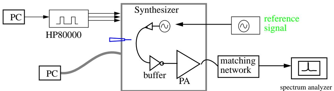
**Fig. 10.19** Setup of PA and Transmitter Testing
