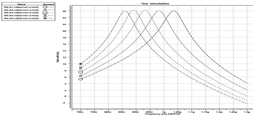
**Fig. 5.8** Frequency Tuning Capability with Re-tuned Q
