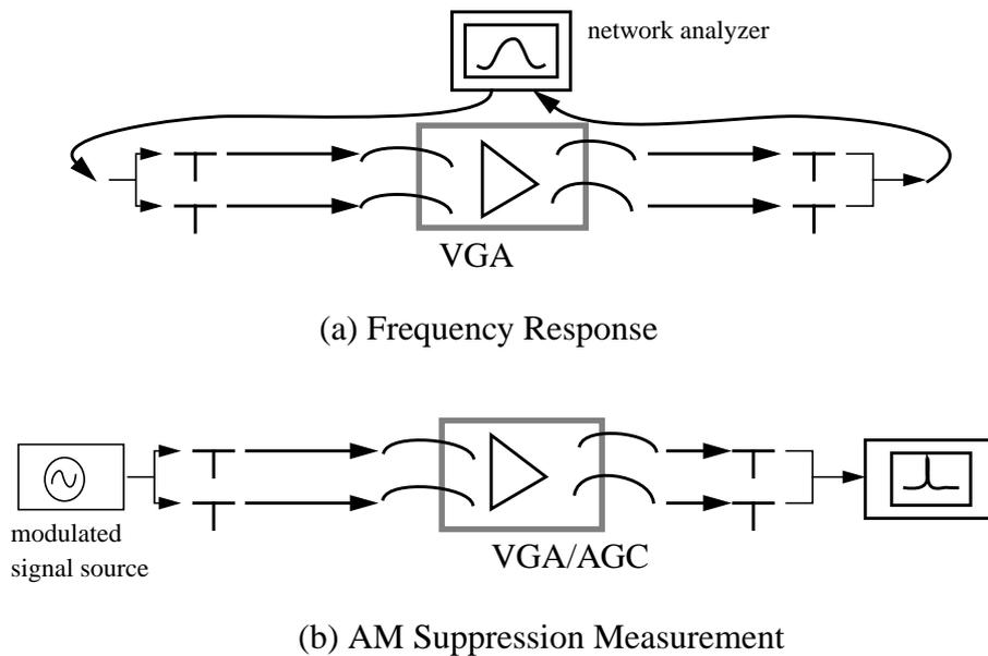
**Fig. 10.16** Setup of VGA Testing
