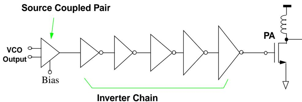
**Fig. 8.7** Buffer driving the PA
