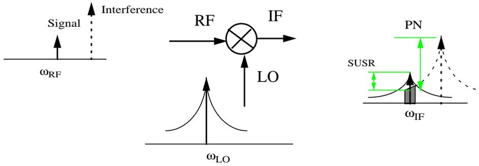
**Fig. 2.6** SNR Degradation due to Phase Noise of the LO Signal
