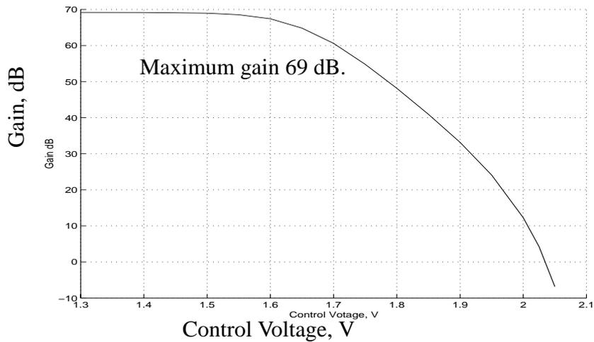
**Fig. 7.5** Simulated VGA Gain-Control Range
