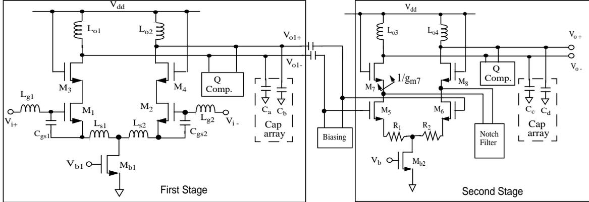
Fig. 5.1 Schematic of the Proposed LNA
