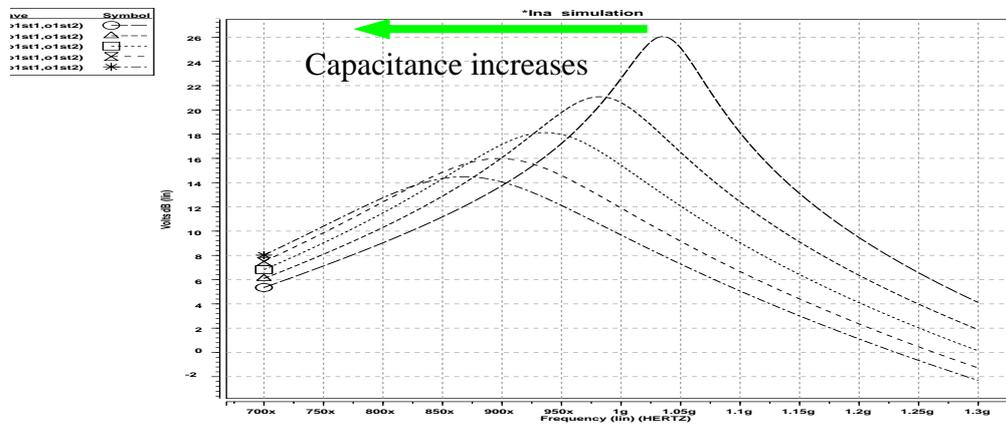
**Fig. 5.7** Frequency Tuning Capability of LNA 1st Stage
