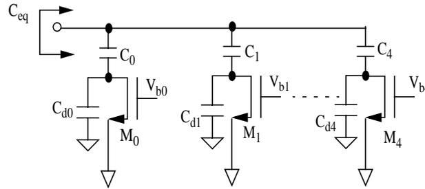
**Fig. 4.4** Switched-Capacitor Array
