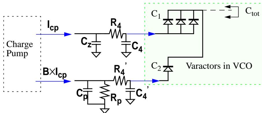
Fig. 6.2 Dual-Path Loop Filter with Signal Added in Capacitance Domain
