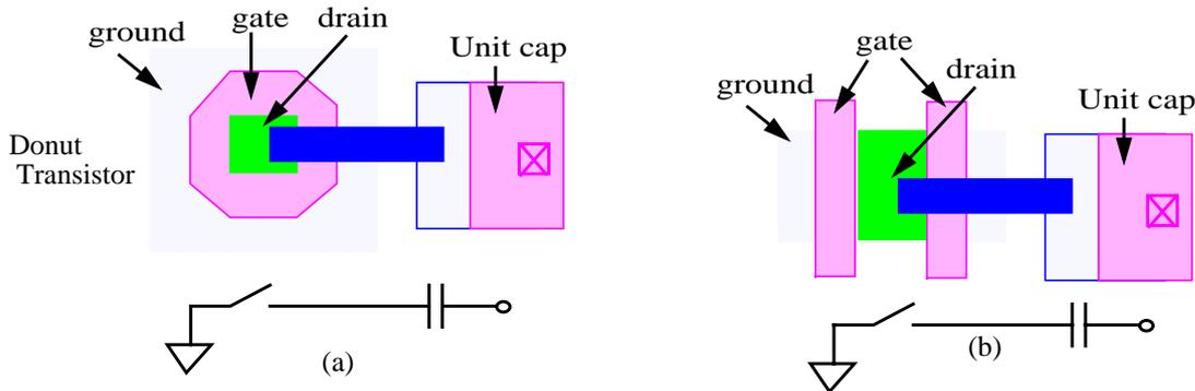
**Fig. 4.5** (a) Donut Transistor and Unit-Cap, (b) Traditional Transistor and Unit-Cap
