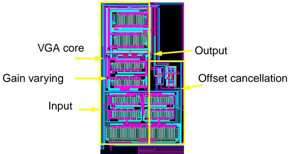
**Fig. 10.6** Layout of each stage of the VGA
