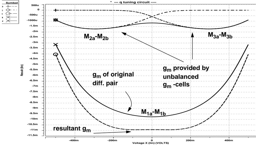
Fig. 5.6  $-G_m$  Curves With and Without Unbalanced  $g_m$ -cells
