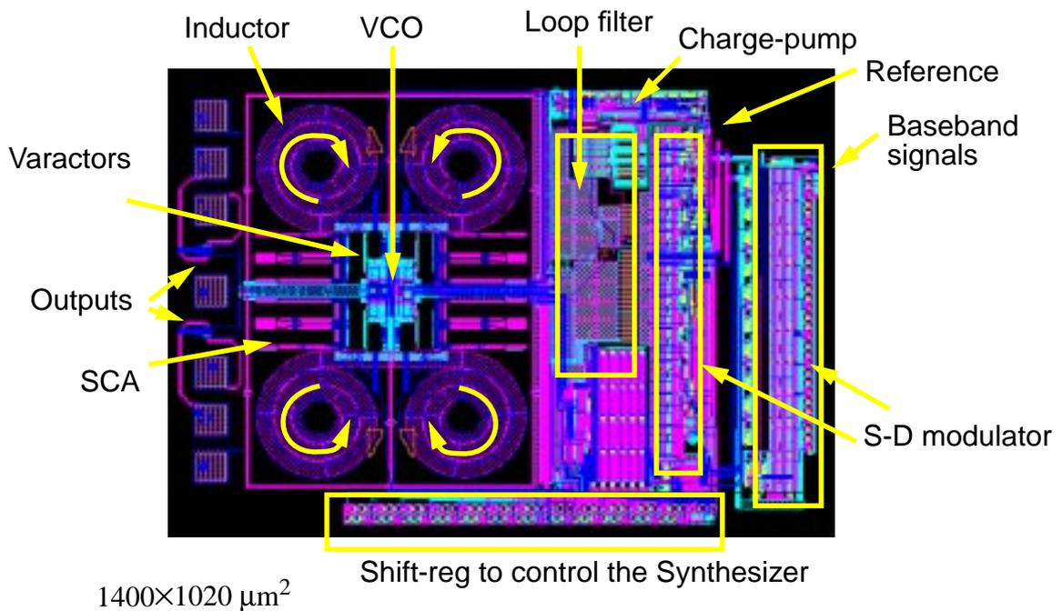
**Fig. 10.5** Layout of the Synthesizer in the Transceiver
