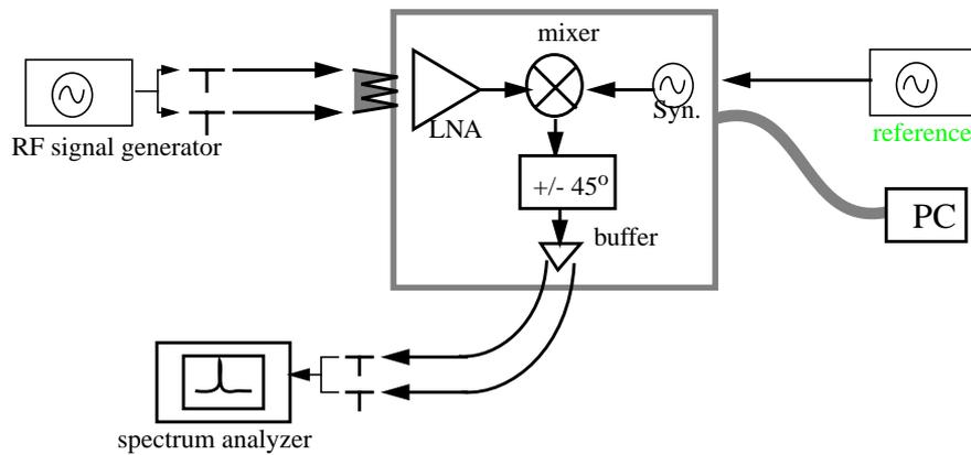
**Fig. 10.14** Setup of RF Front-End Testing
