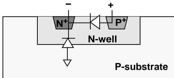
**Fig. 4.6** Parasitic PN Junction Varactor
