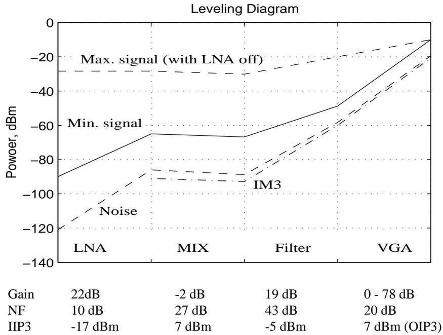
Fig. 10.37 Signal-level diagram of the proposed receiver
