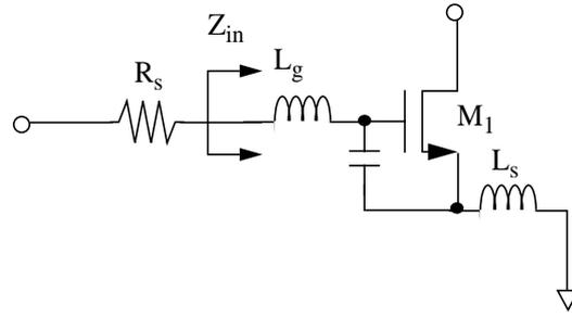
**Fig. 5.2** Inductive Degeneration Used as Input Matching
