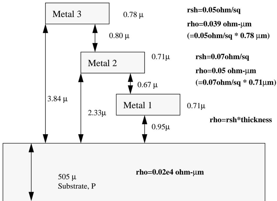
Fig. 4.2 Process information of a Typical 0.5μm CMOS
