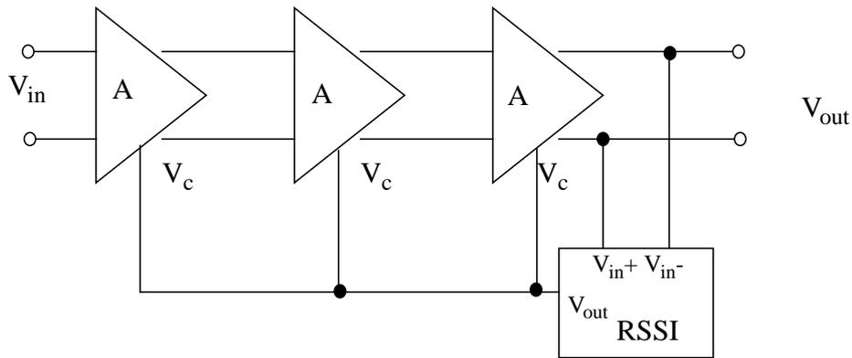
**Fig. 7.10** Block Diagram of the AGC Loop
