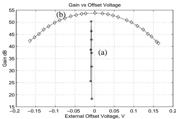
**Fig. 10.32** VGA Gain Variation due to Offset Voltage
