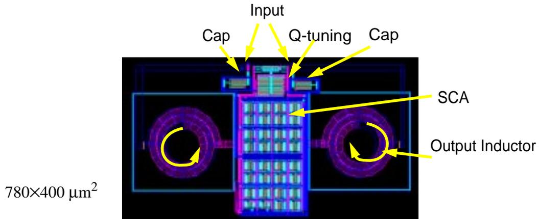
**Fig. 10.4** Layout of the Notch Filter in the Receiver
