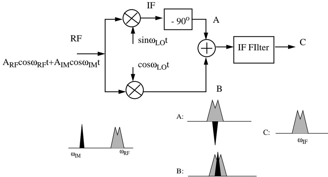
**Fig. 2.4** I-Q Downconverter to Remove Image Signal
