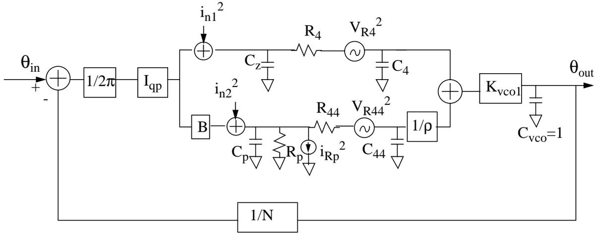
Fig. 6.6 Behavior Model with the Noise Sources
