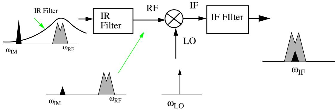
**Fig. 2.3** Image Rejection Filter to Remove Image Signal
