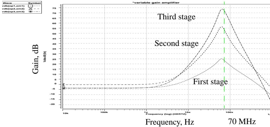
**Fig. 7.8** The Simulated Frequency Response of The VGA with Offset Cancellation
