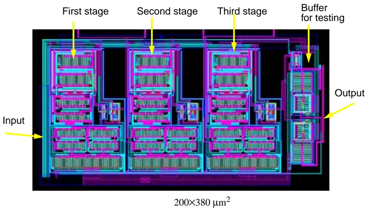
**Fig. 10.7** Layout of the whole VGA
