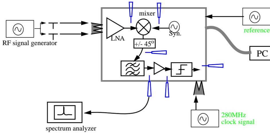
**Fig. 10.18** Setup of Receiver Testing
