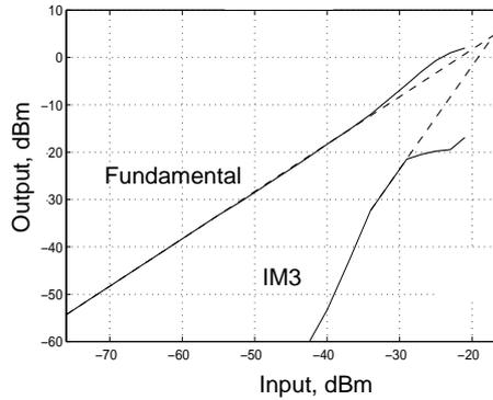
**Fig. 10.22** Two-Tone Measurement of the LNA
