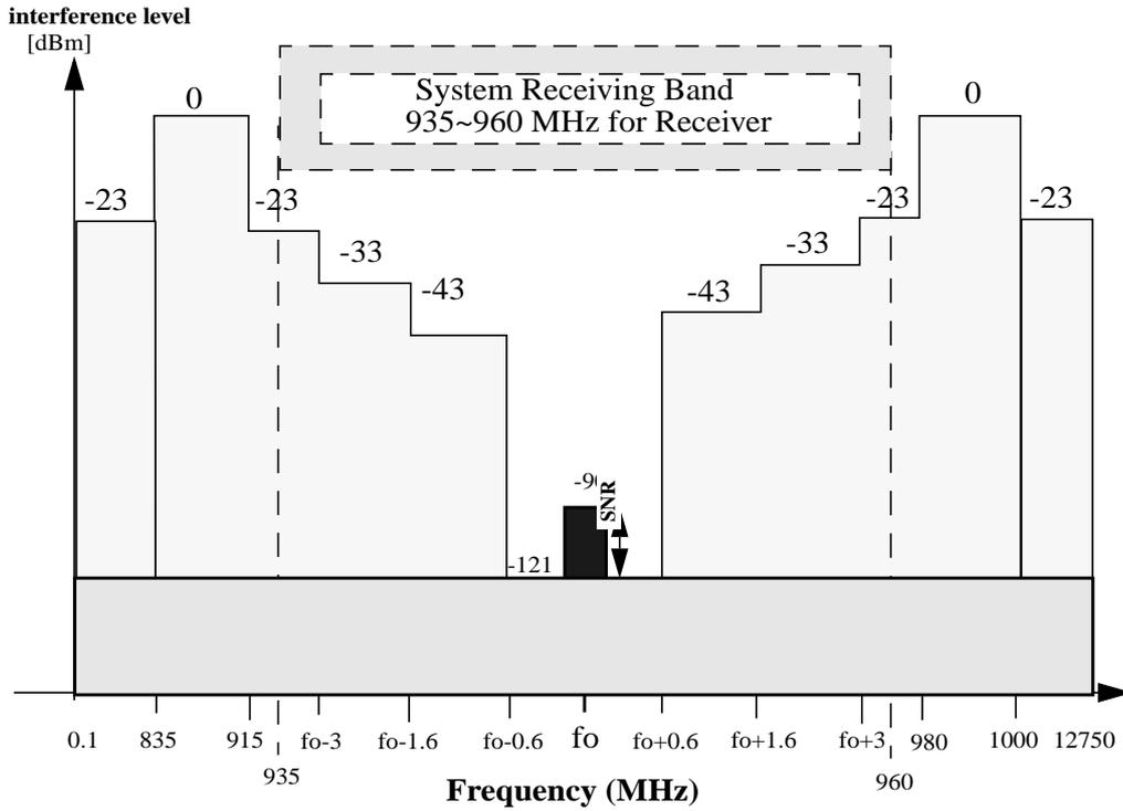
**Fig. 3.4** Specifications of Blocking Signals
