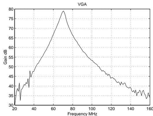
**Fig. 10.30** Frequency Response of the VGA
