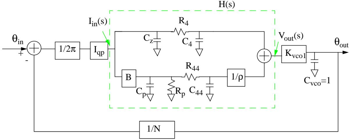
**Fig. 6.4** Behavior Model of the Synthesizer
