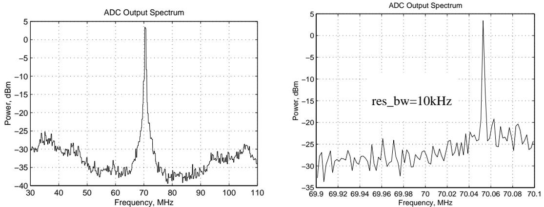
Fig. 10.36 Measured output spectrum of the whole receiver with a -90-dBm input to LNA
