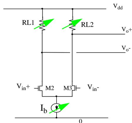
**Fig. 7.1** Existing Gain Varying Techniques
