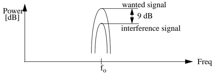
Fig. 3.2 Cochannel Interferences
