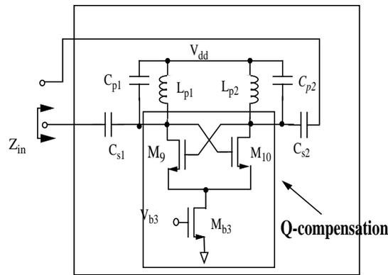
Fig. 5.9 Schematic of the Proposed Notch Filter
