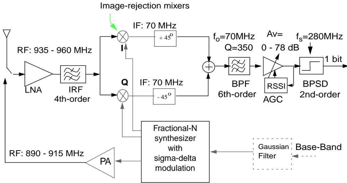
**Fig. 3.8** Proposed Transceiver
