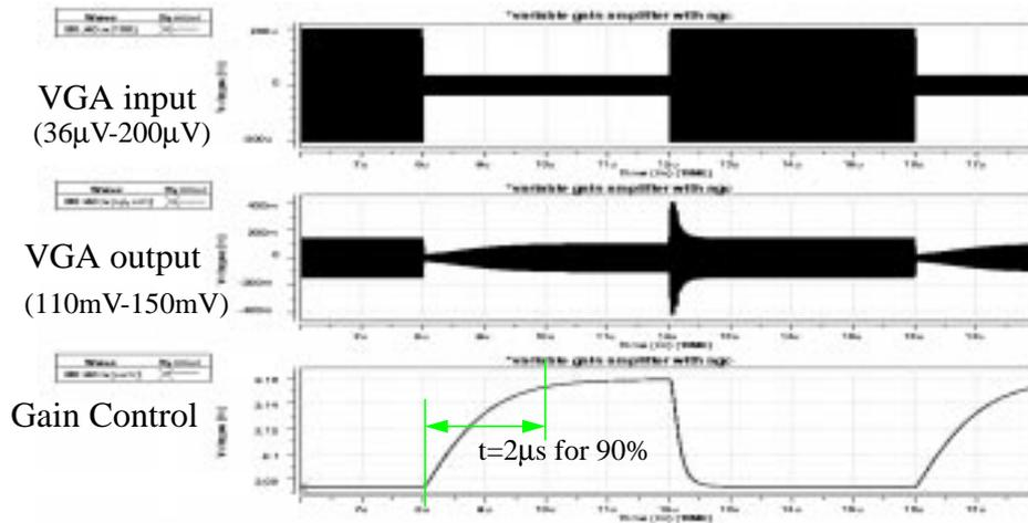
**Fig. 7.11** Transient Simulation of the AGC Loop
