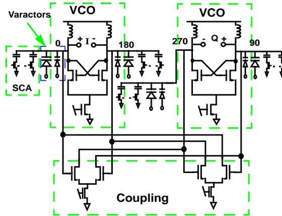
Fig. 6.3 VCO with Switched-Capacitor Array
