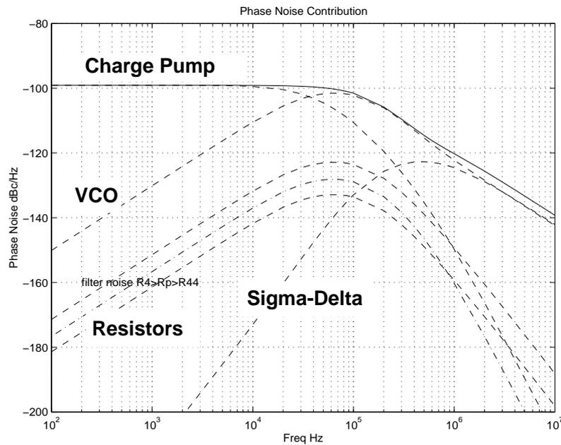
**Fig. 6.7** Phase Noise Contribution of Each Noise Source
