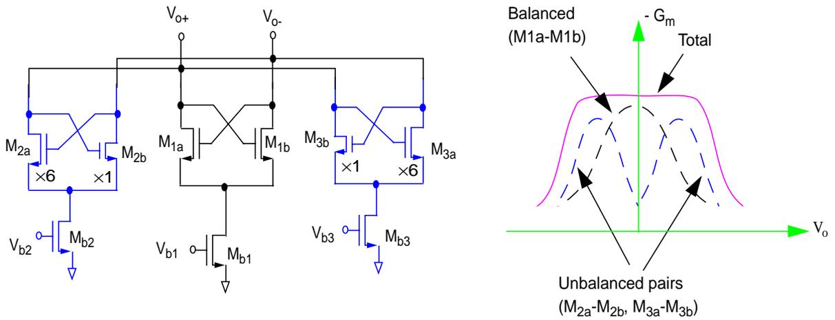
**Fig. 5.5** Unbalanced  $-G_m$  of the Proposed Q-Compensation Circuit
