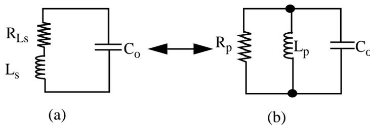
Fig. 5.4 Equivalent Parallel Resonant Circuit for the Output
