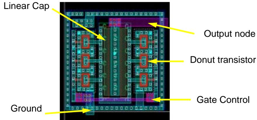
**Fig. 10.2** Layout of Double-Unit-Caps Used in the LNA
