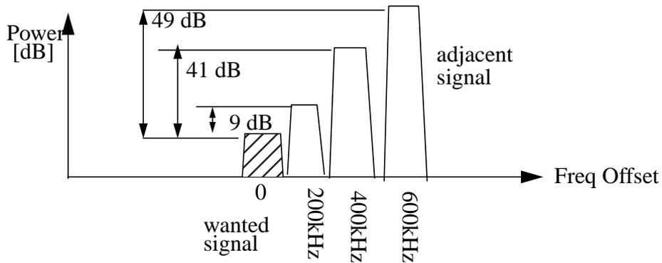
Fig. 3.3 Adjacent Channel Interference
