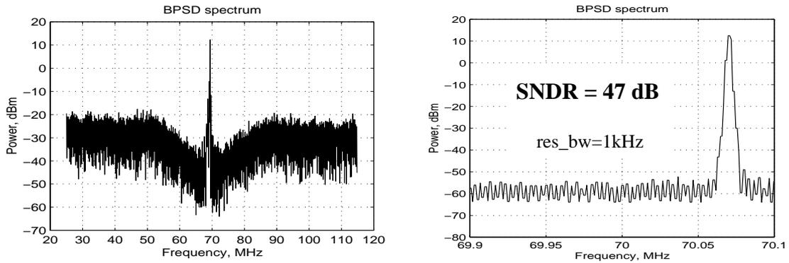
Fig. 10.35 Output Spectrum of the BPSD ADC
