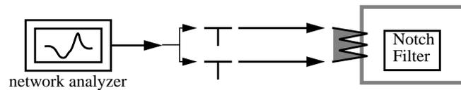
**Fig. 10.12** Setup of Notch Filter Testing
