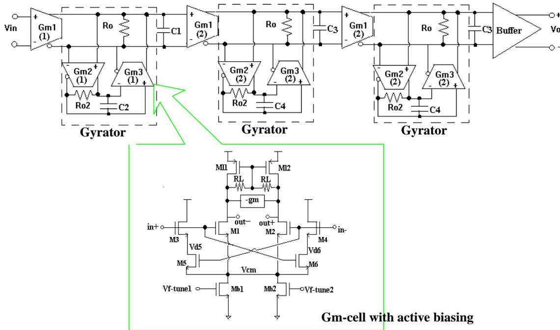
**Fig. 8.3** Circuit implementation of the channel-selection IF filter
