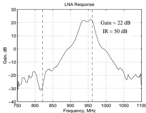
**Fig. 10.21** Frequency Response of LNA and IRF
