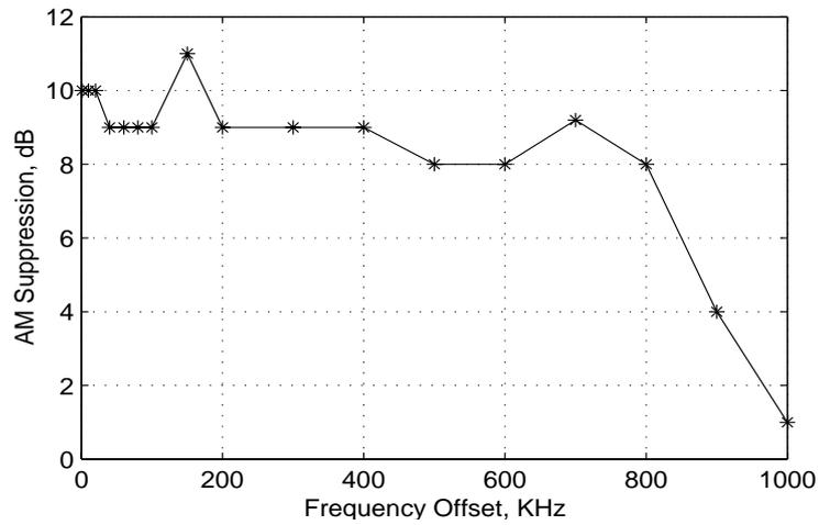
**Fig. 10.34** AM Suppression of the AGC Loop
