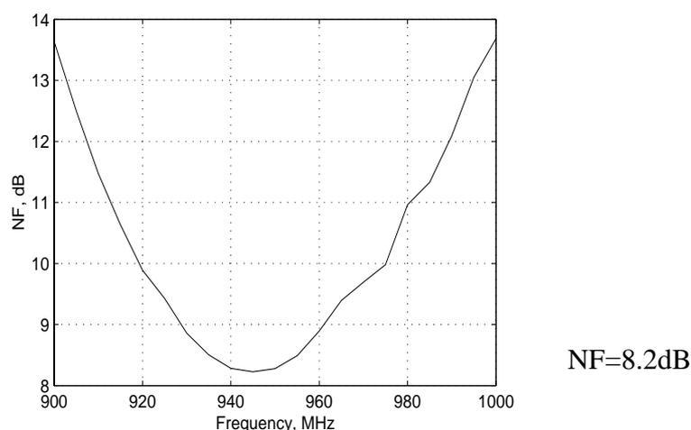
**Fig. 10.24** NF of LNA with Bond-wire Inductors as Gate Inductors
