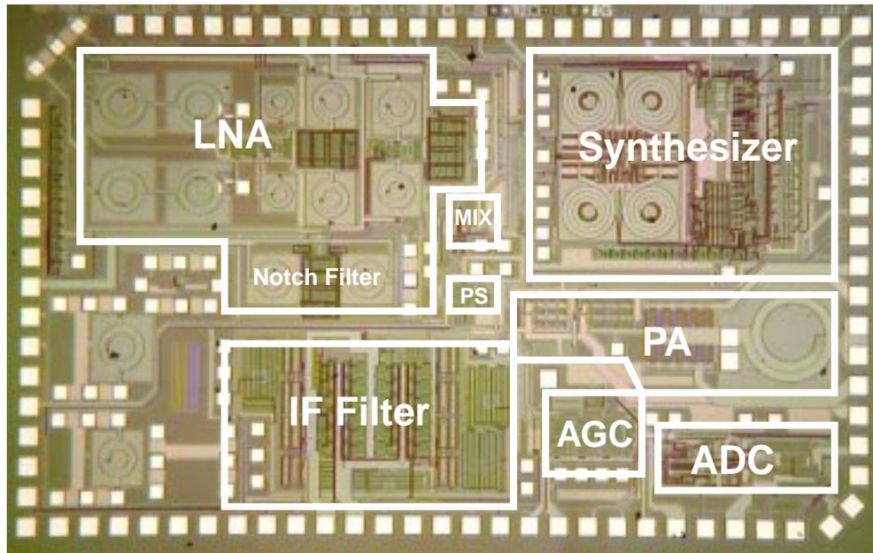
**Fig. 10.10** Die Photo of the Transceiver
