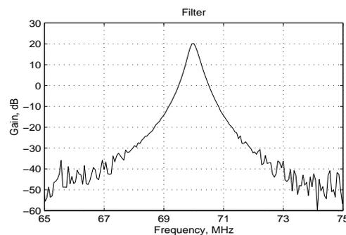
**Fig. 10.28** Frequency Response of the IF Filter
