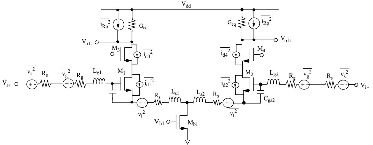
**Fig. 5.12** Equivalent Circuit of LNA with Noise Sources
