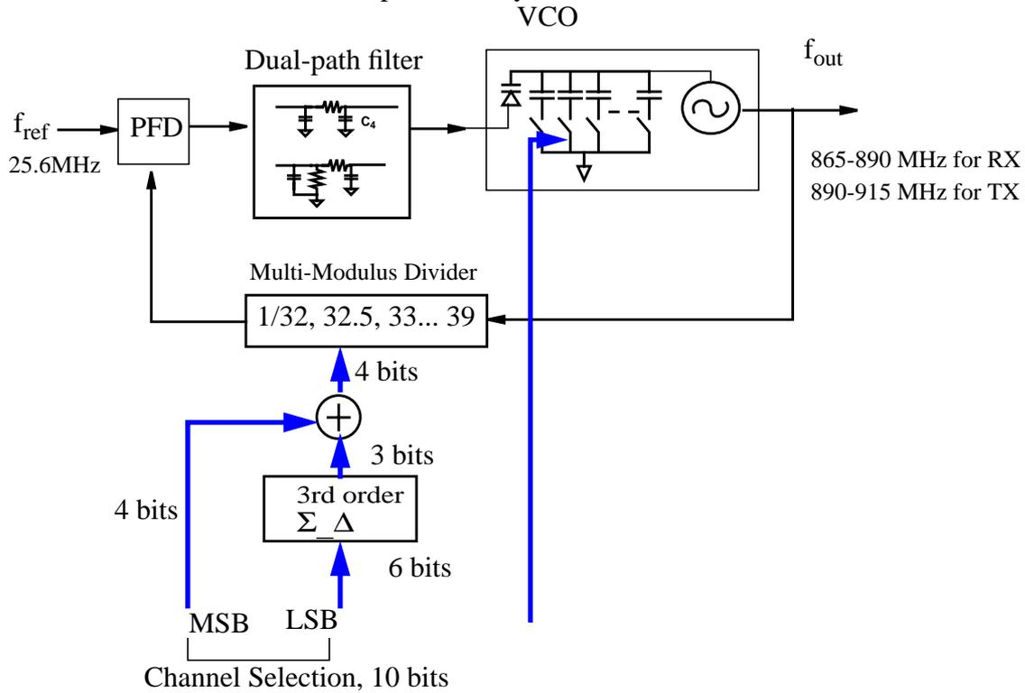
**Fig. 6.1** Proposed Synthesizer with Sigma-Delta Modulation
