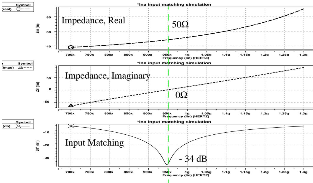
Fig. 5.3 Simulation Result of Input Matching, Single-Ended
