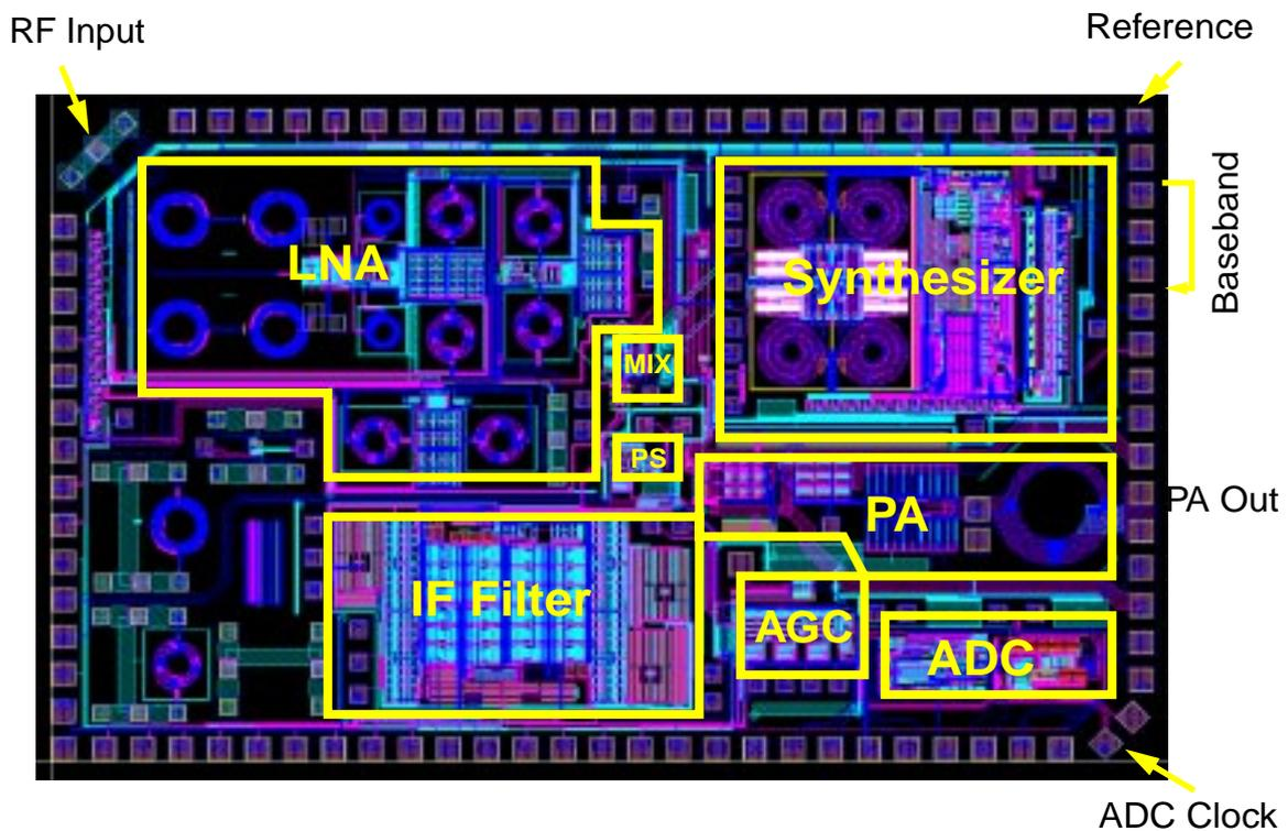
**Fig. 10.9** Layout of Whole Transceiver
