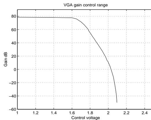
**Fig. 10.31** VGA Gain Control Range
