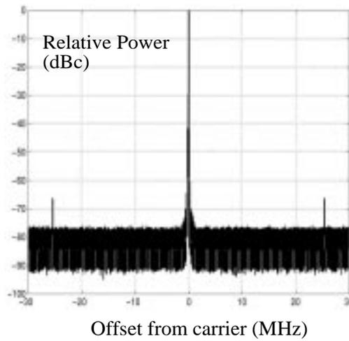
**Fig. 10.26** Output spurs of the synthesizer
