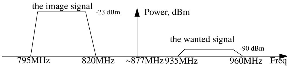
**Fig. 3.9** The Image Signal and the Desired Signal
