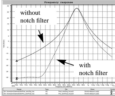
Fig. 5.11 Frequency Response of the LNA With and Without Notch Filter
