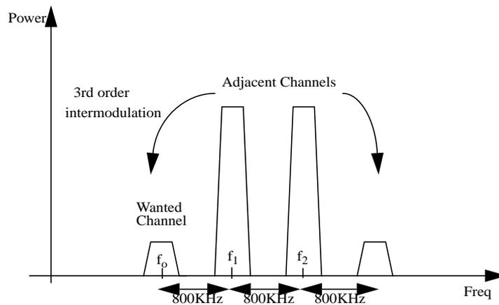
**Fig. 3.5** Degradation of the receiver performance due to intermodulation
