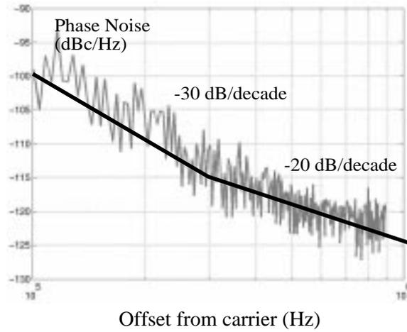
**Fig. 10.25** Measured output phase noise of the synthesizer
