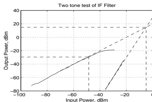
**Fig. 10.29** Two-tone measurement of the IF Filter
