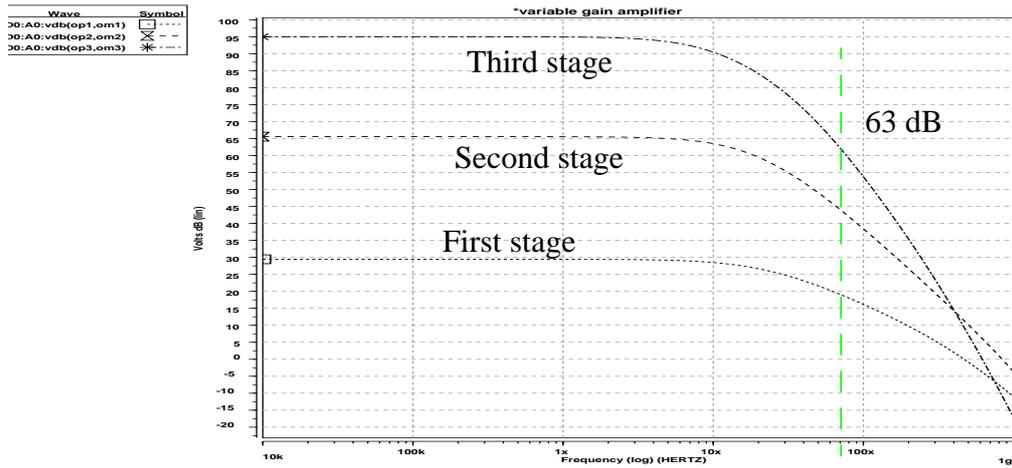
**Fig. 7.4** Simulated VGA Frequency Response
