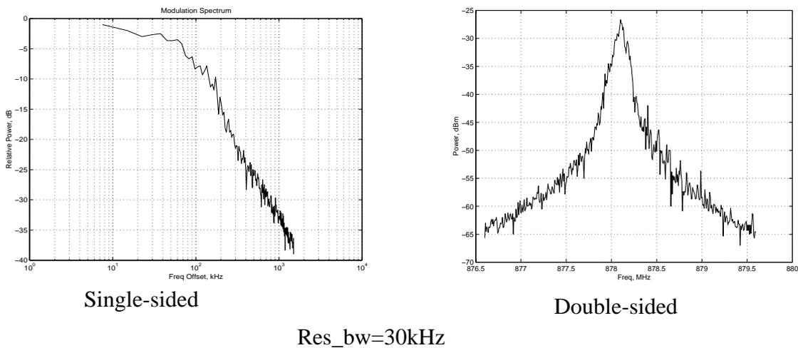
Fig. 10.38 Modulated RF Spectrum
