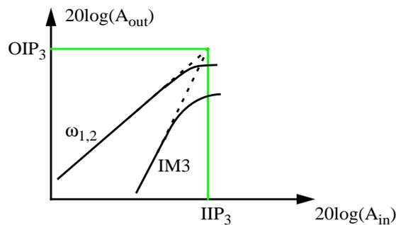
**Fig. 2.1** Two-tone Test of a Nonlinear System
