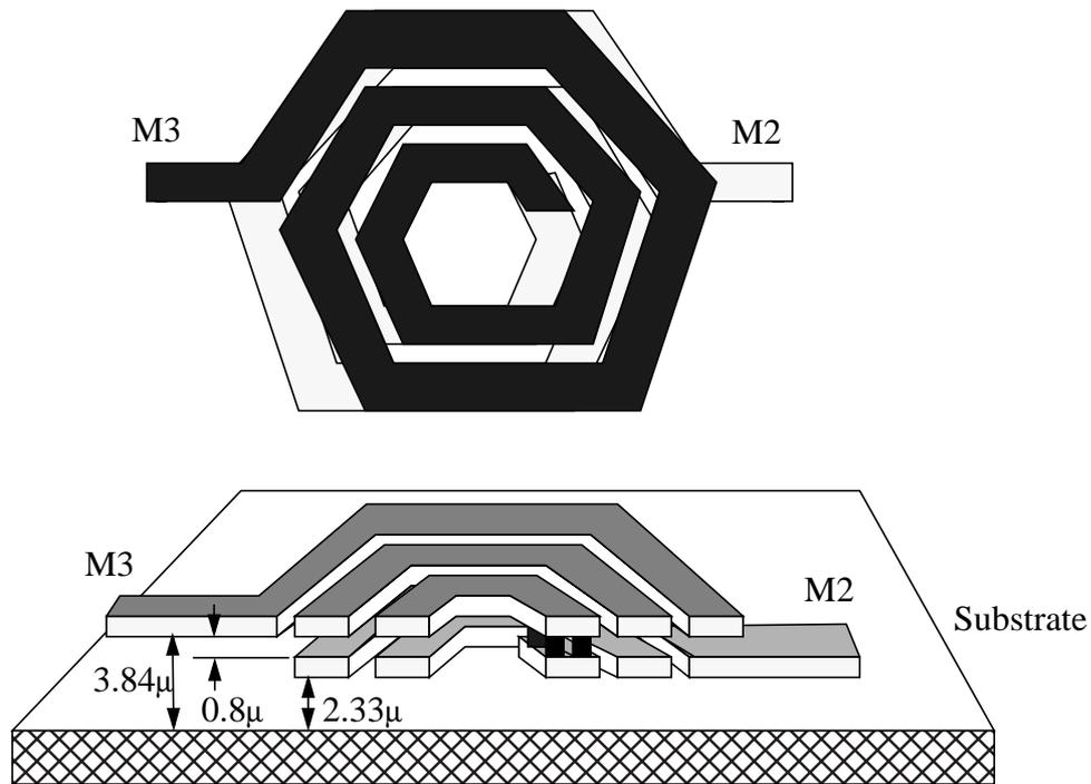
**Fig. 4.3** Double-layer On-Chip Inductor
