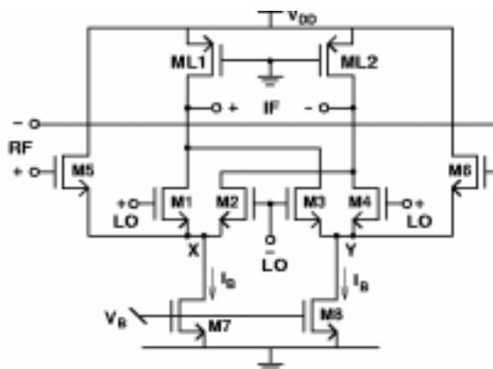
**Fig. 8.1** Circuit schematic of the mixer
