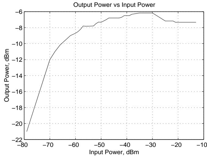
**Fig. 10.33** AGC Input Power and Output Power
