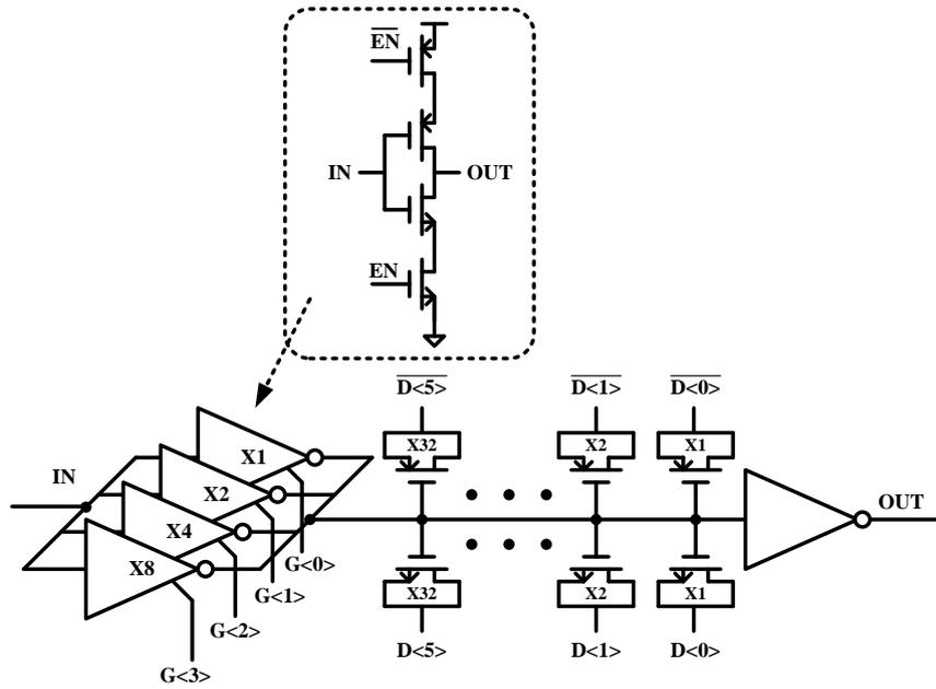
Fig. 5. 8 fine segment of the phase modulator
