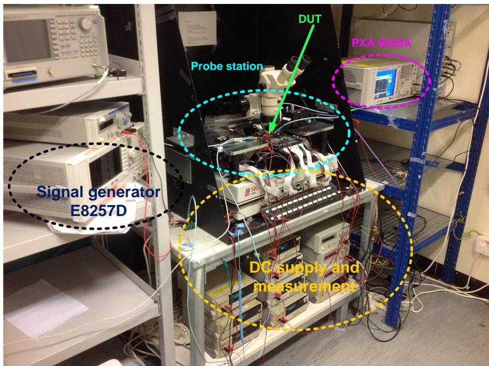
Fig. 7. 3 Measurement setup for the all digital polar transmitter
