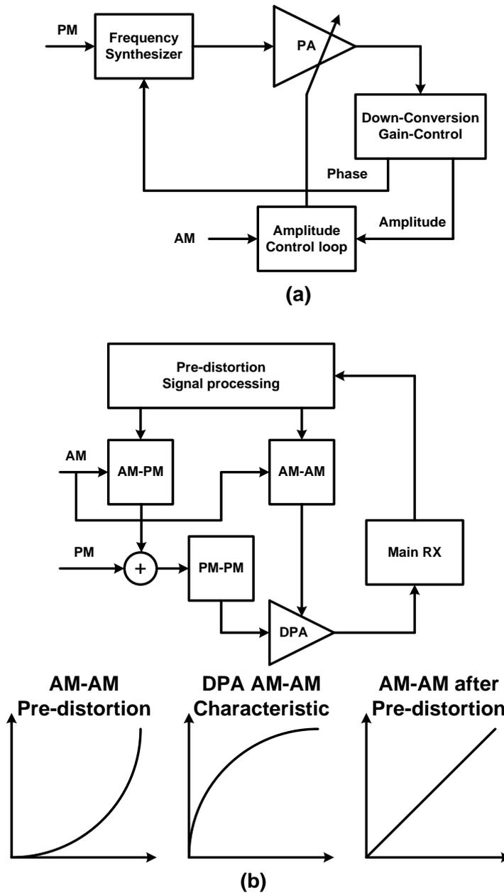
Fig. 6. 2 existing transmitter linearization techniques (a) close-loop transmitter and (b) digital pre-distortion
