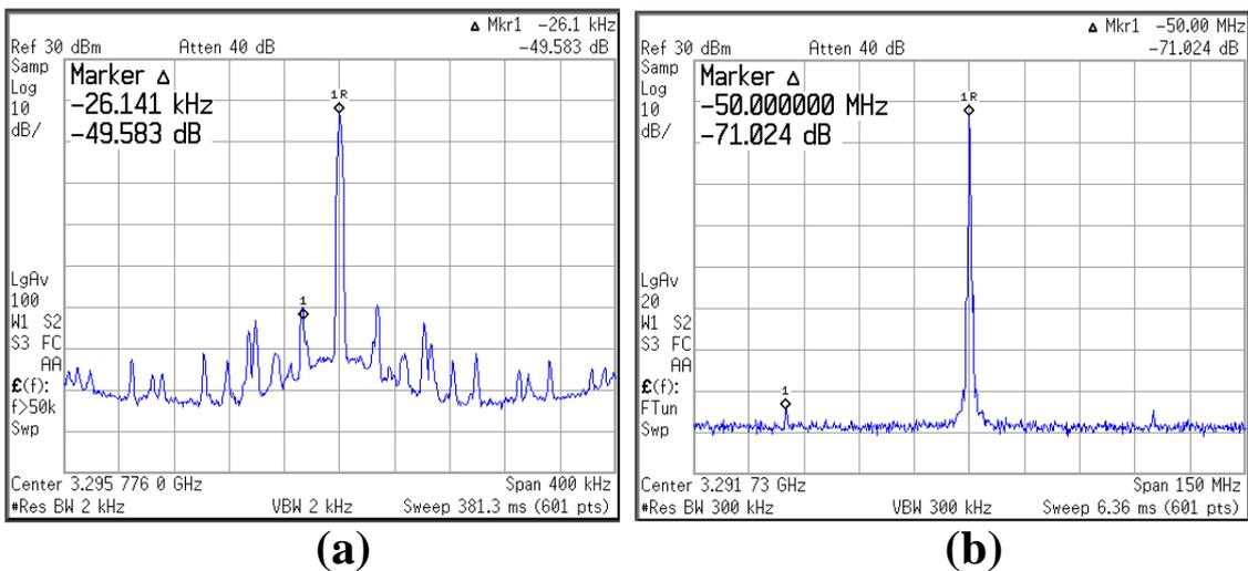
Fig. 3. 39 Measured ADPLL spurs (a) in-band fractional spurs and (b) reference spurs
