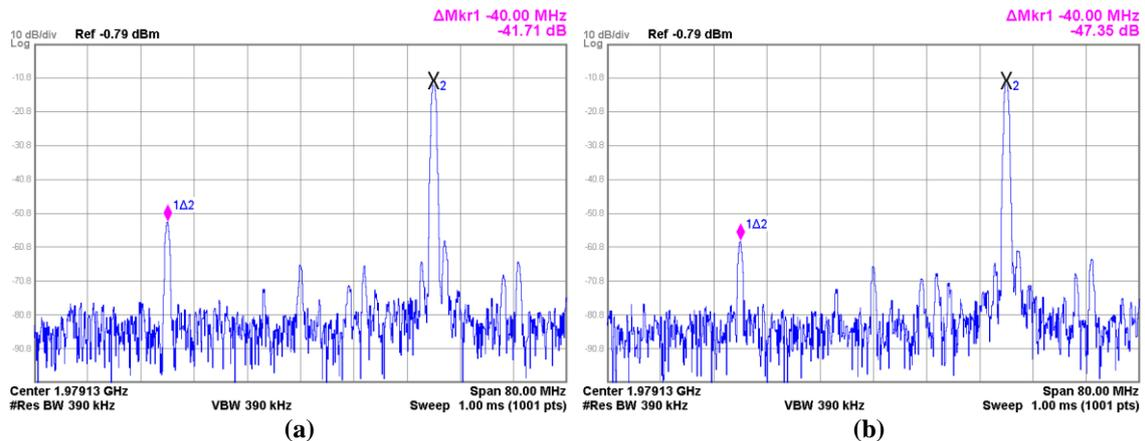
Fig. 7. 11 Measured quadrature error of  $\pm 1.5$  divider (a) without DCC and (b) with DCC
