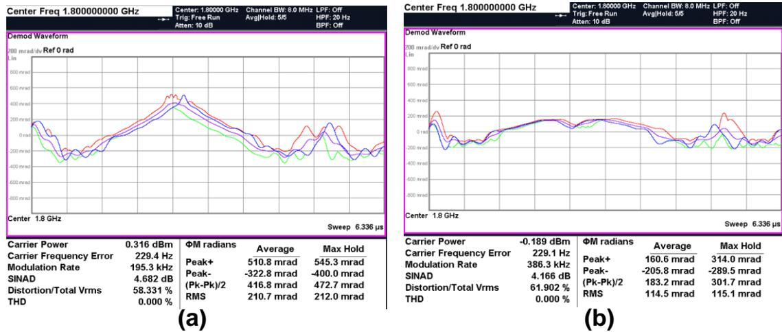
Fig. 7. 16 PA AM-PM (a) without linearization (b) with linearization
