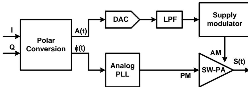
Fig. 2. 11 Traditional polar transmitter architecture
