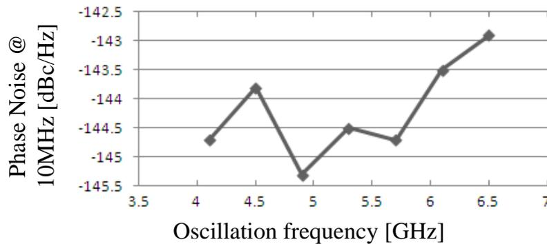
Fig. 3. 12 Measured phase noise at 10MHz offset frequency across the entire frequency tuning range
