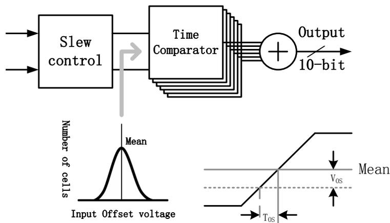
Fig. 3. 19 Statistical TDC with gain control
