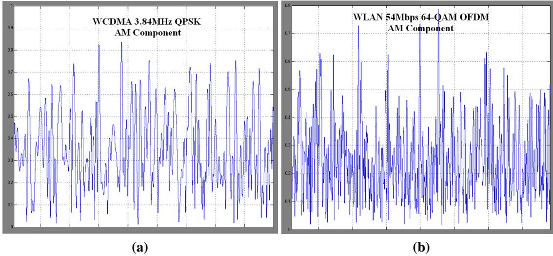
Fig. 2. 5 The AM component of (a) WCDMA and (b) WLAN signals
