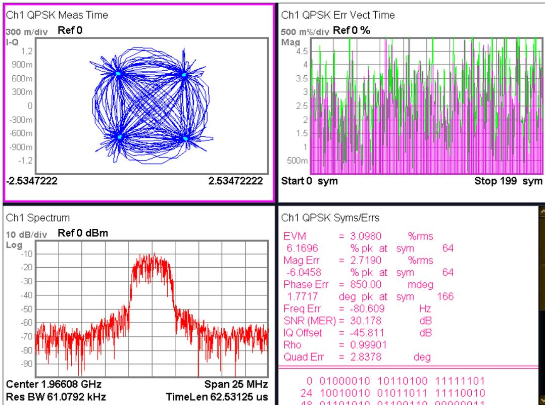
Fig. 7. 18 Measured WCDMA spectral mask and EVM
