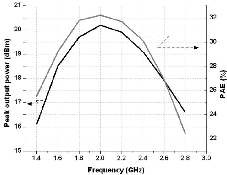
Fig. 6. 15 Measured peak output power and PAE as functions of the RF frequency
