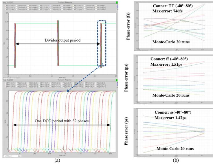
Fig. 3. 32Simulation result of the 32-phase interpolator (a) 32-phase output waveform and (b) phase error under different conditions
