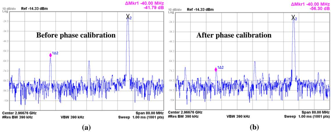
Fig. 7. 6 QDCO quadrature error measurement (a) before phase calibration (b) after phase calibration
