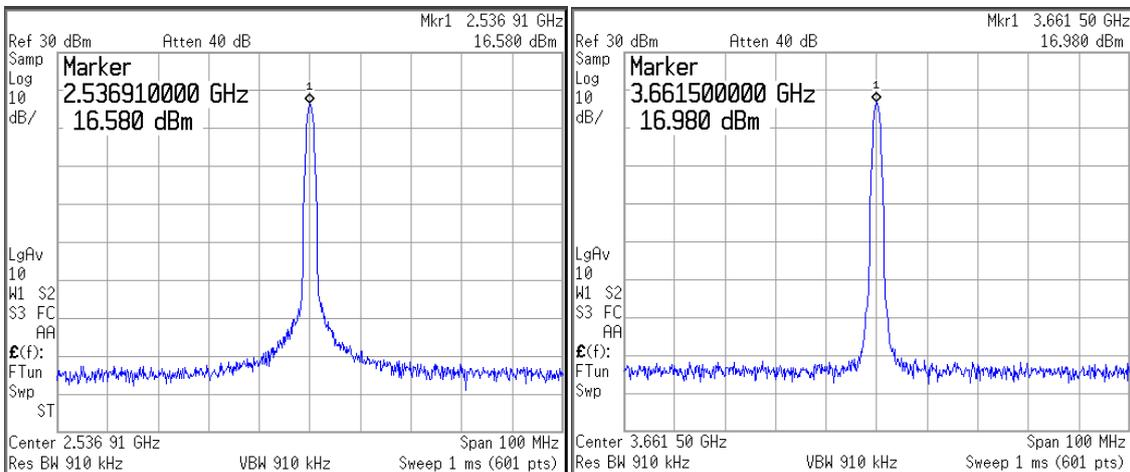
Fig. 7. 4 QDCO output frequency range
