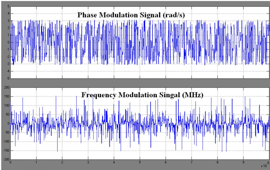
Fig. 5. 4 PM components of a WLAN 54Mbps 64-QAM OFDM transmitted signal
