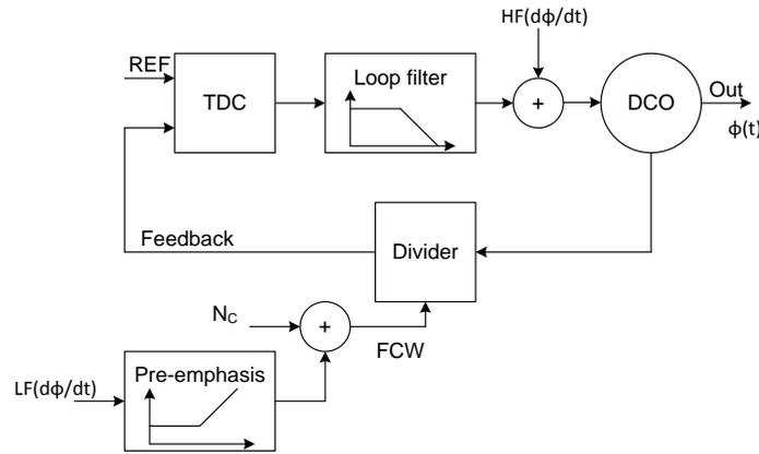
Fig. 5. 3 Block diagram of an ADPLL for the wide-band PM
