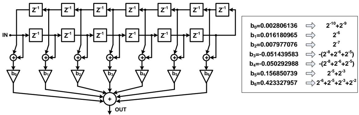
Fig. 6. 13 Implementation of the first-stage FIR filter
