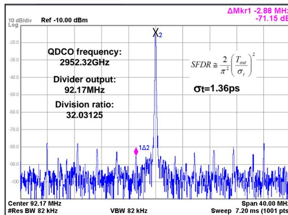
Fig. 3. 33 The measured output spectrum of the sub-integer divider
