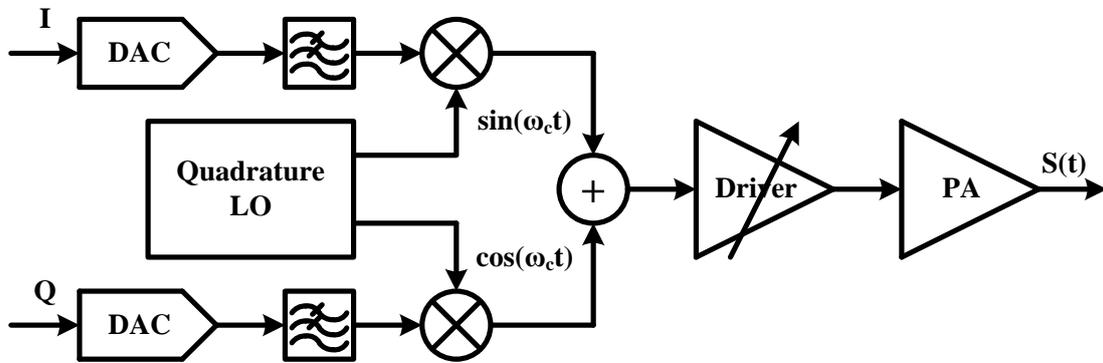
Fig. 2. 9 Block diagram of the direct conversion transmitter
