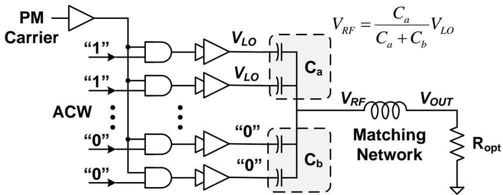
Fig. 6. 5 Block diagram of the SCPA [6.17]
