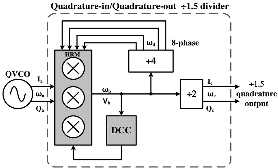
Fig. 4. 7 block diagram of the proposed Quadrature-in/Quadrature-out  $\div 1.5$  divider
