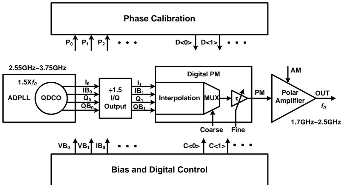
Fig. 7. 1 System block diagram of the digital polar transmitter
