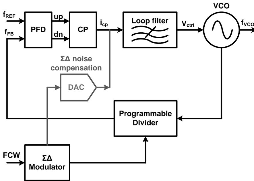
Fig. 3. 2 Block diagram of an analog PLL
