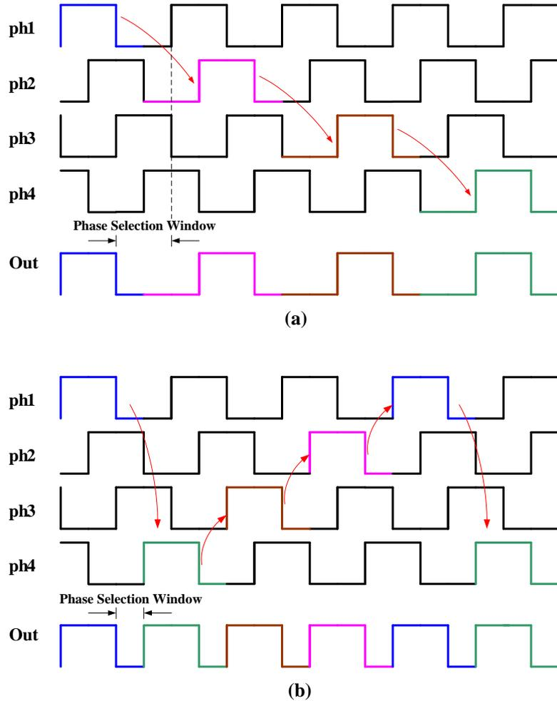
Fig. 4. 3 Phase-Rotating Frequency Division (a) divide by 1.25 and (b) divide by 0.75
