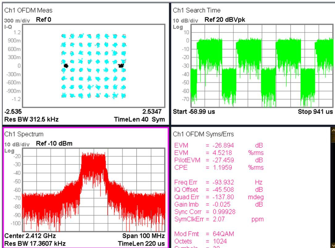
Fig. 7. 20 Measured spectral mask and EVM for WLAN 802.11g 54-Mb/s 64-QAM OFDM data
