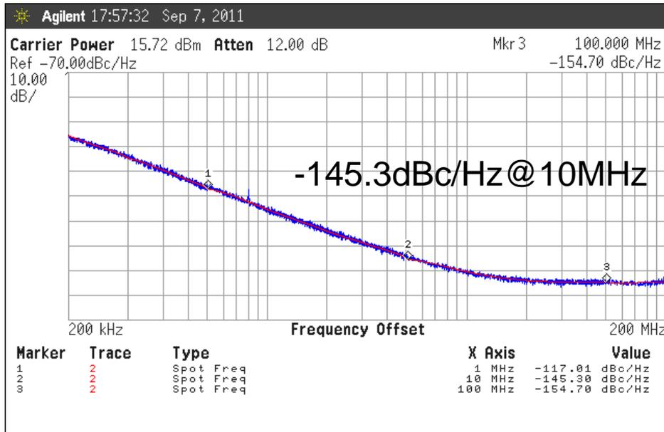
Fig. 3. 11 QDCO phase noise measure at 4.9GHz
