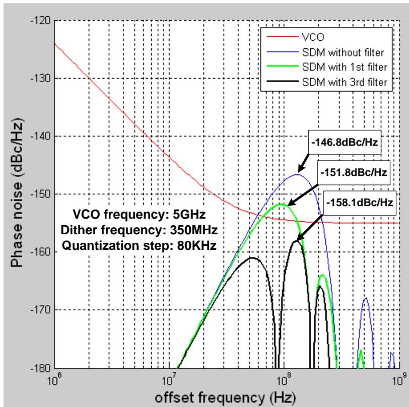
Fig. 3. 10 Phase noise simulation of the proposed QDCO
