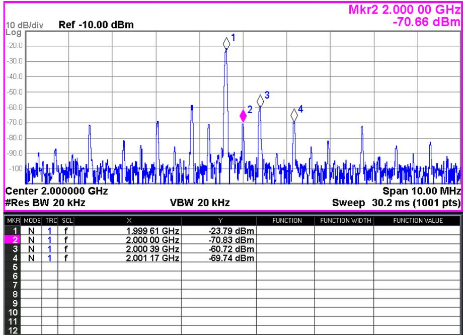
Fig. 7. 13 PM linearity measurement
