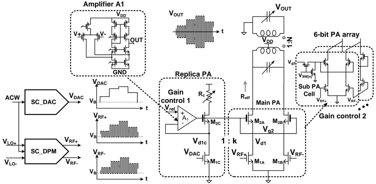
Fig. 6. 8 Schematic of the proposed PA with AM replica linearization
