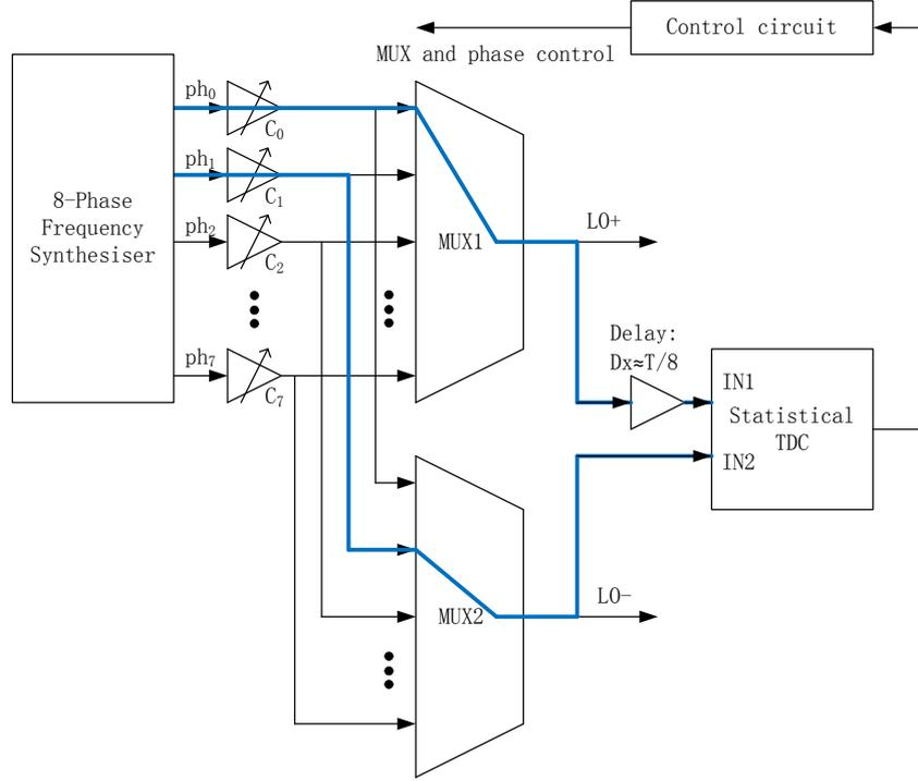
Fig. 5. 9 Blocks diagram of the phase selection and calibration
