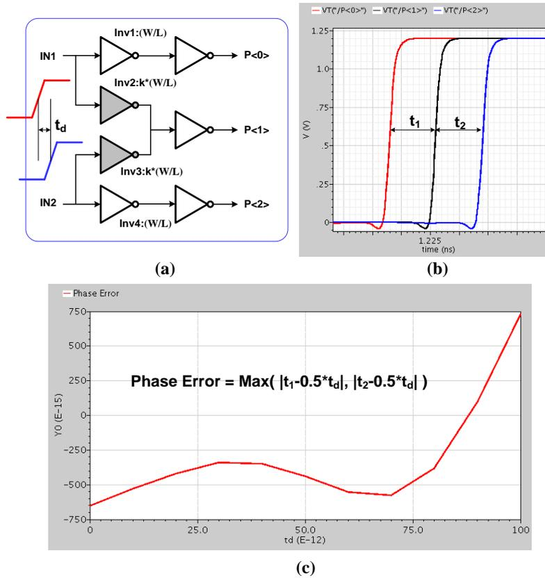
Fig. 3. 31 Phase interpolator (a) simplify implementation, (b) Transient simulation and (c) Simulation of the Phase Error
