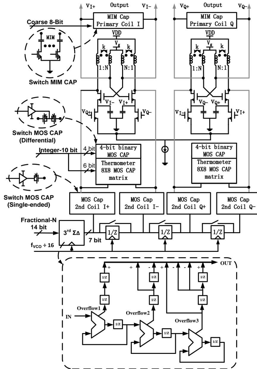
Fig. 3. 8 Schematic of the proposed QDCO with  $\Sigma\Delta$  shaped quantization noise filter
