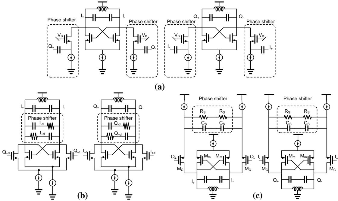
Fig. 3. 5 existing QVCO with phase shifter (a) Common gate amplifier as the phase shifter, (b) phase shifter in the tank, and (c) phase shifter with buffer and RC filter
