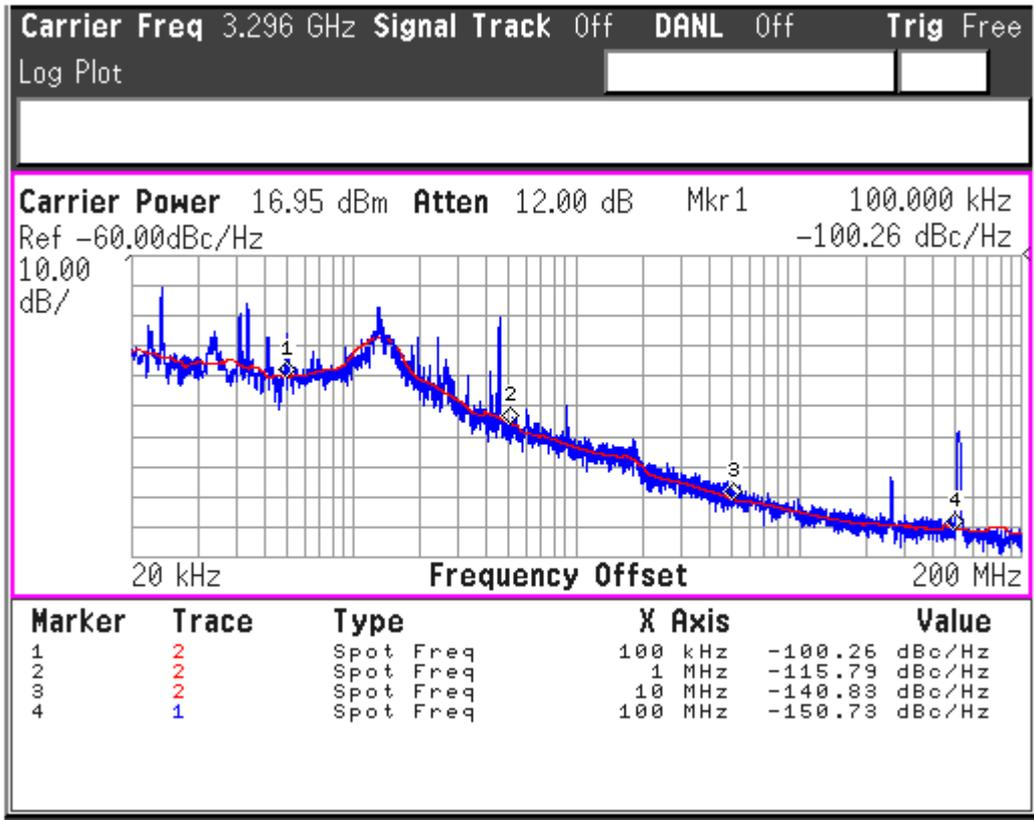
Fig. 3. 38 The measured phase noise of the ADPLL
