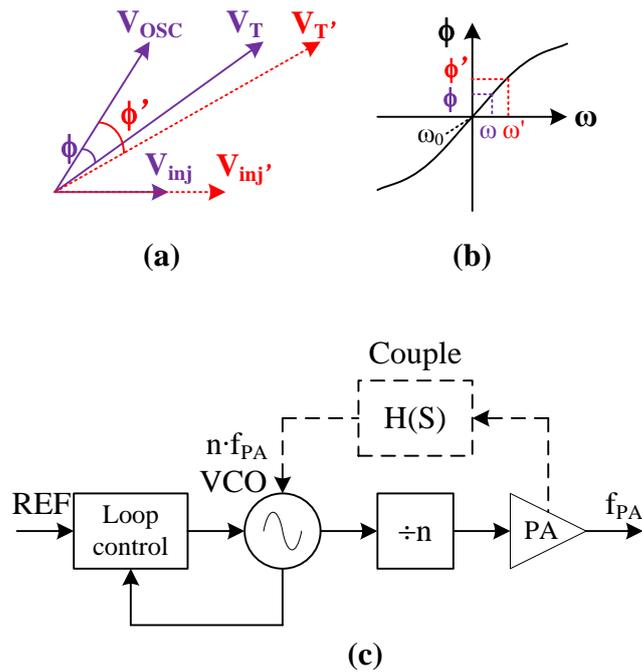
Fig. 4. 1 LO pulling mechanism (a) Phasor representation of signals in the VCO (b) Phase response of the resonance tank (c) Block diagram of the LO pulling mechanism
