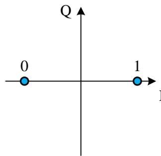
Fig. 2. 2 constellation diagram example for BPSK
