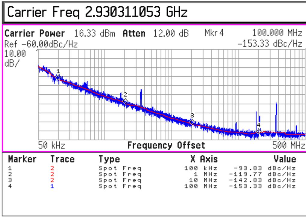
Fig. 7. 5 QDCO output phase noise
