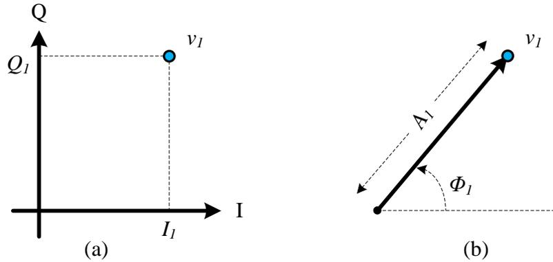
Fig. 2. 1 two views of a vector signal space (a) I-Q projections (b) polar form
