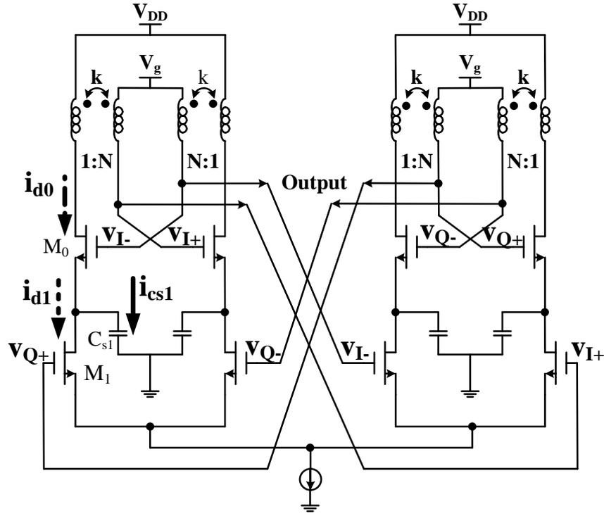
Fig. 3. 6 Proposed Class-C QVCO with phase shifters
