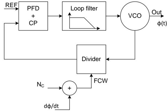
Fig. 5. 1 Block diagram of PLL based PM
