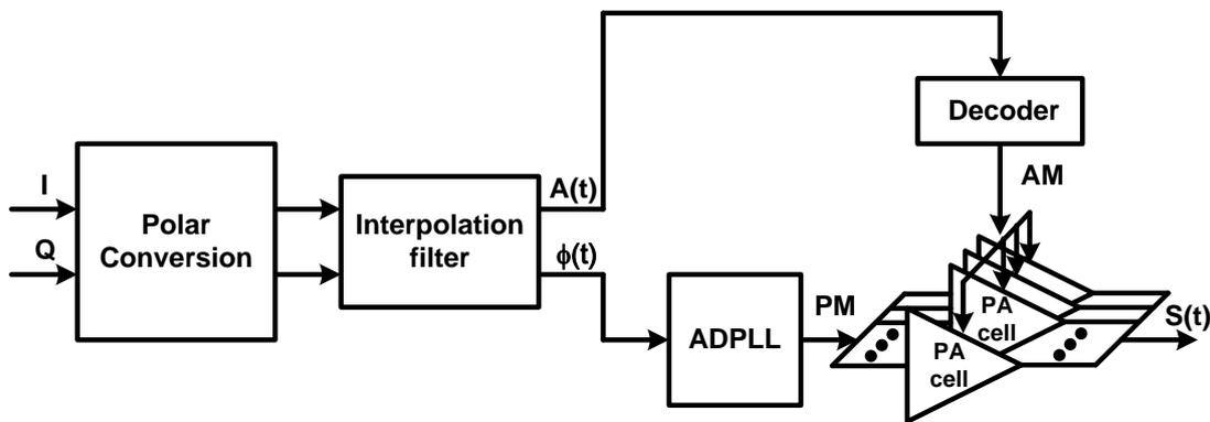
Fig. 2. 12 All-digital polar transmitter architecture
