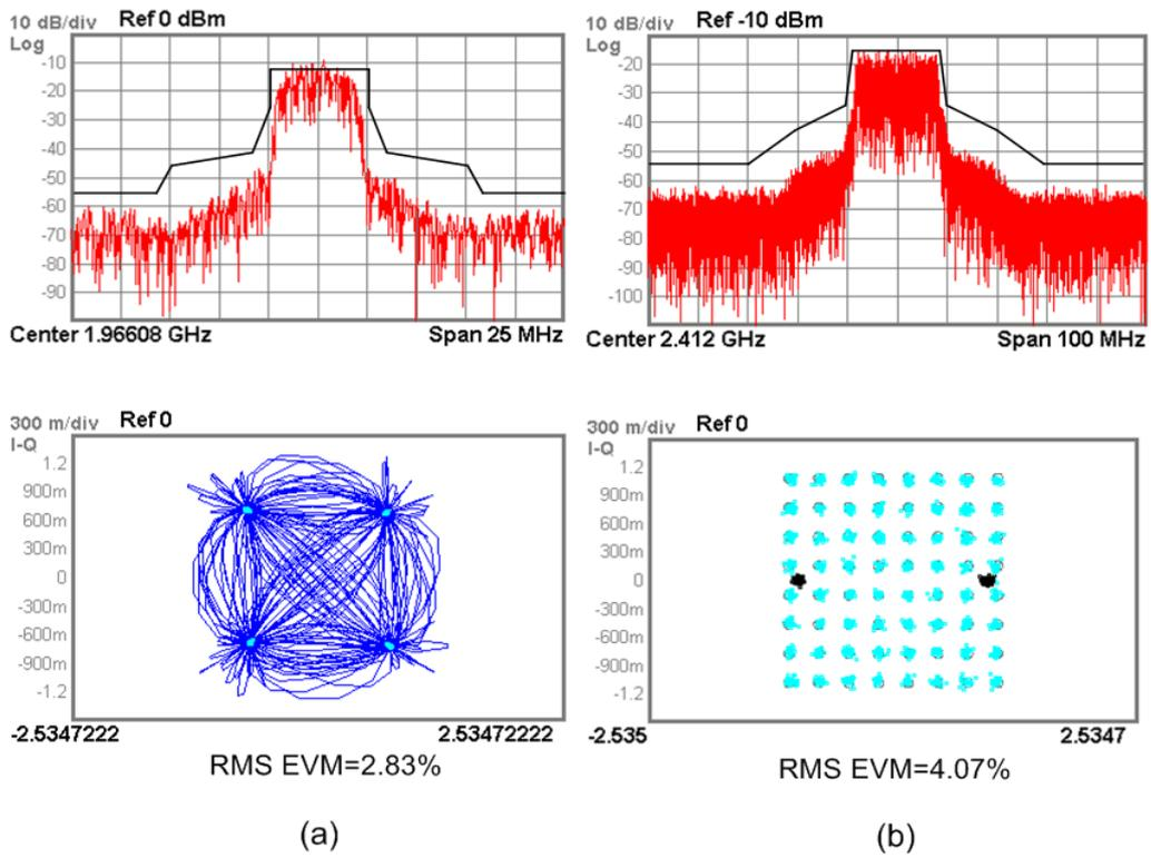
Fig. 6. 16 Measured spectral mask and EVM for: (a) WCDMA, and (b) WLAN 802.11g 54-Mb/s 64-QAM OFDM data
