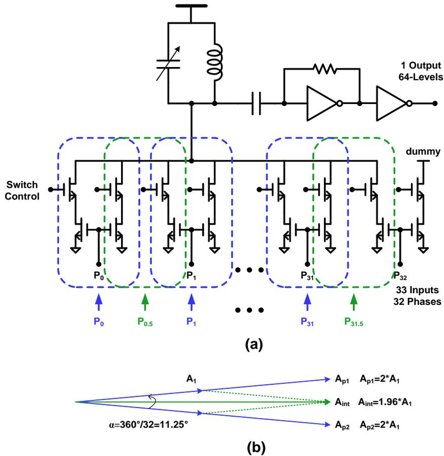
Fig. 5. 7 64-phases selection MUX (a) Implementation and (b) amplitude mismatch
