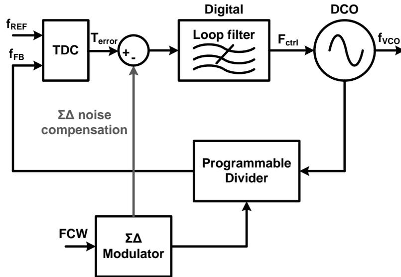
Fig. 3. 3 Block diagram of the ADPLL
