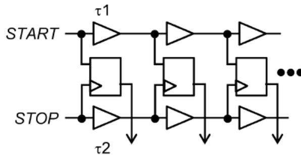
Fig. 3. 17 Vernier delay line based TDC
