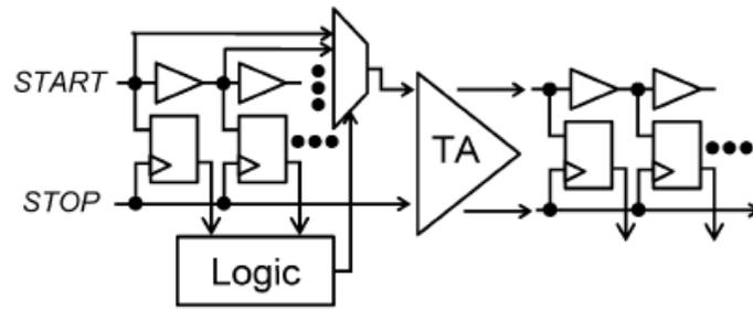
Fig. 3. 18 Two-step TDC with time amplifier
