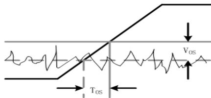
Fig. 3. 25 TDC noise due to the noise of the time comparator
