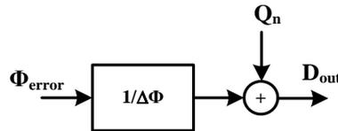
Fig. 3. 16 Linear model of the TDC
