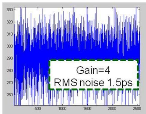
Fig. 3. 26 Measured TDC output with a fixed input
