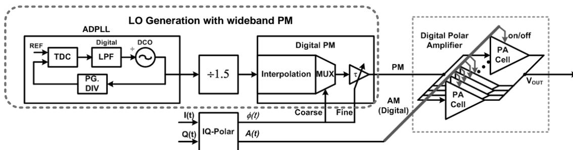
Fig. 2. 14 Proposed all digital polar transmitter architecture
