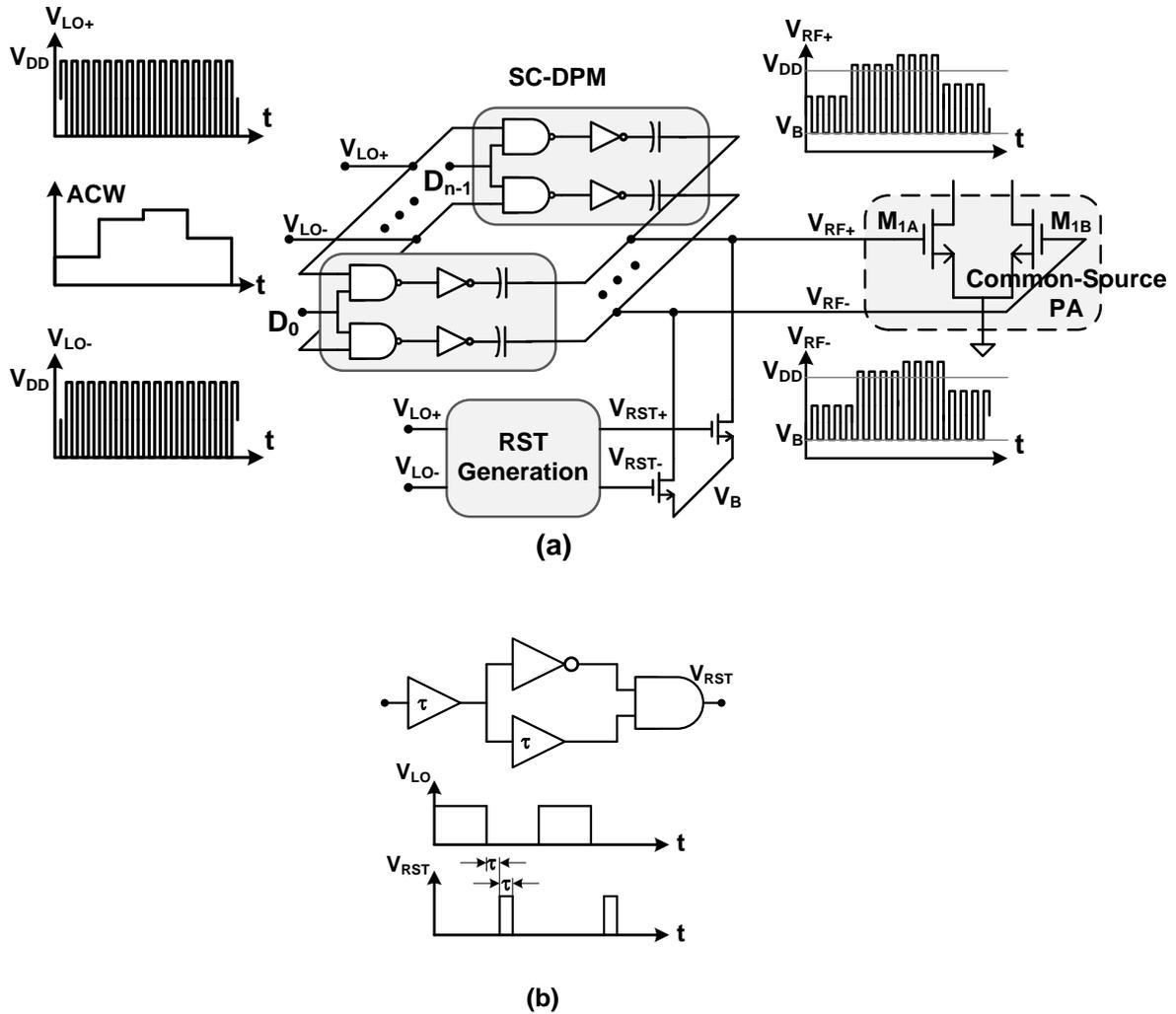
Fig. 6. 6 Block diagram of (a) the proposed SC-DPM, and (b) its RST generation circuit
