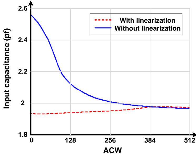
Fig. 6. 11 Simulated PA input capacitance versus ACW
