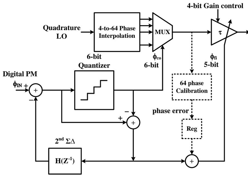
Fig. 5. 5 proposed phase interpolated digital phase modulator
