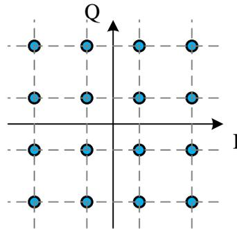
Fig. 2. 4 constellation diagram example for 16-QAM
