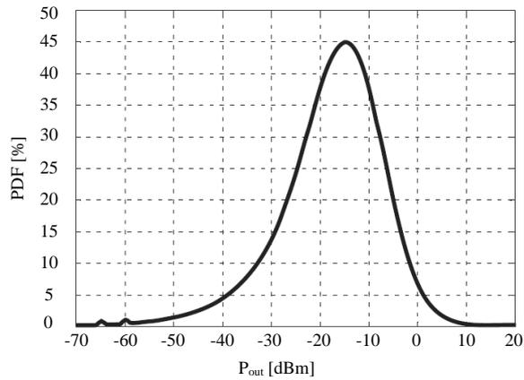
Fig. 2. 6 PDF versus output power of the WCDMA mobile station transmitter
