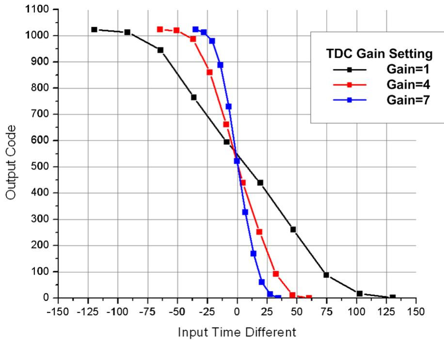
Fig. 3. 23 Measured TDC input-output characteristic with different slew rate
