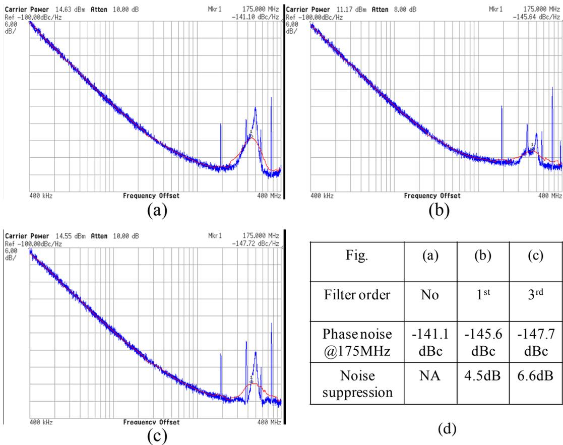
Fig. 3. 13 QDCO out-band phase noise measurements: (a)  $\Sigma\Delta$  modulator turns on without filter, (b)  $\Sigma\Delta$  modulator turns on with 1st-order filter, and (c)  $\Sigma\Delta$  modulator turns on with 3rd-order filter (d) Summary of the performance
