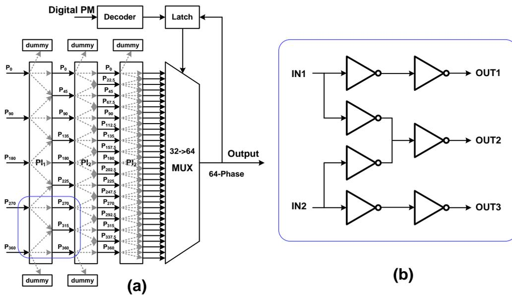
Fig. 5. 6 coarse segment of the phase modulator (a) Block diagram and (b) PI-cell
