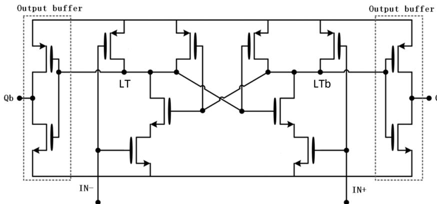
Fig. 3. 21 Time comparator for the TDC
