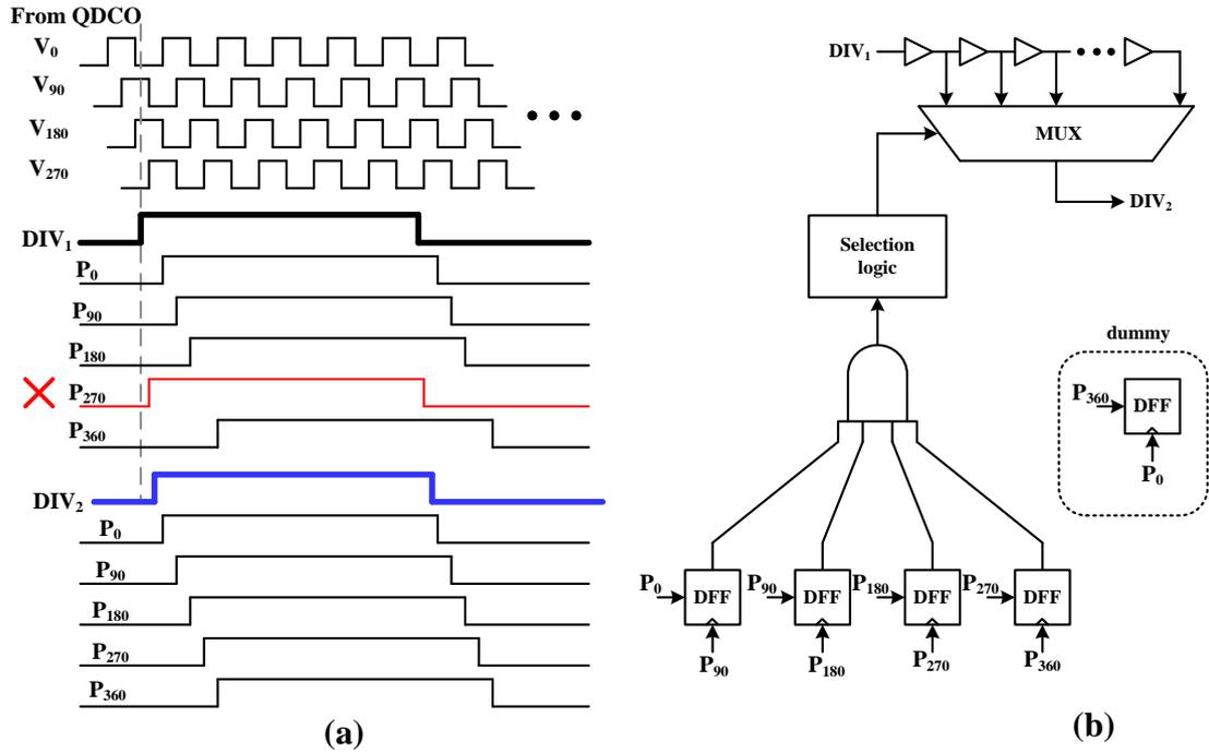
Fig. 3. 30 Phase sequence correction (a) timing diagram (b) circuit implementation
