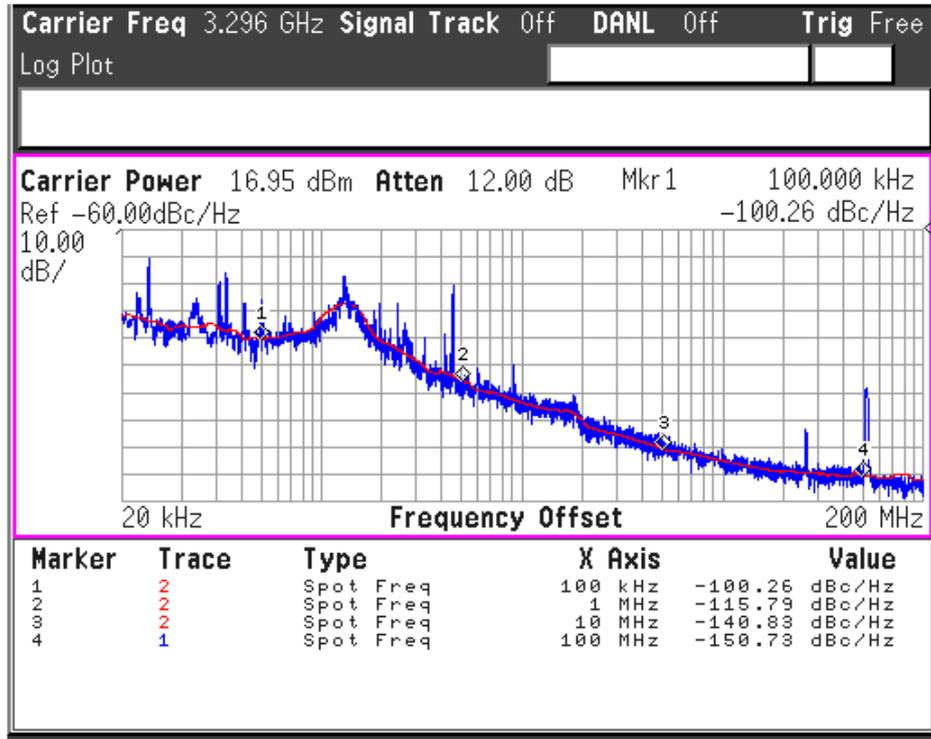
Fig. 7. 8 The measured phase noise of the ADPLL
