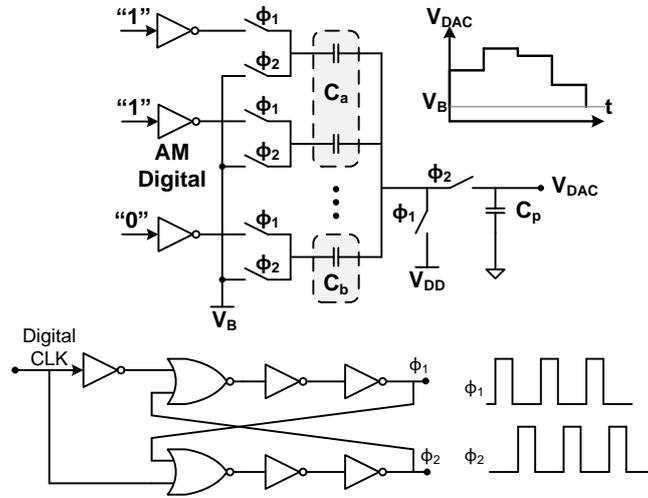
Fig. 6. 7 Schematic of the proposed SC-DAC circuit
