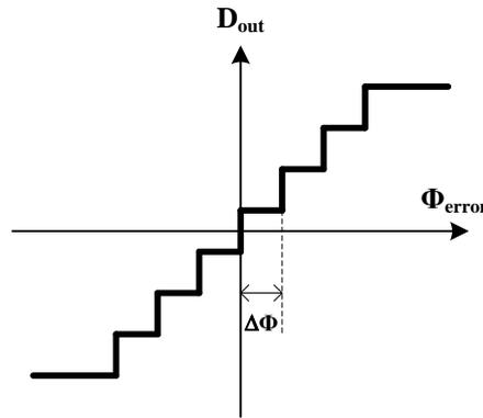
Fig. 3. 15 Transfer characteristic of the TDC
