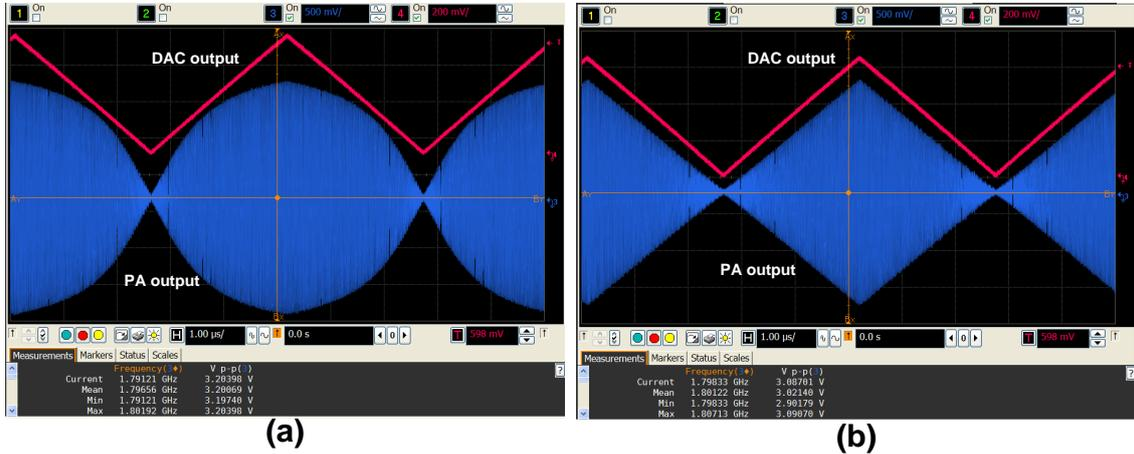
Fig. 7. 15 PA AM-AM (a) without linearization (b) with linearization
