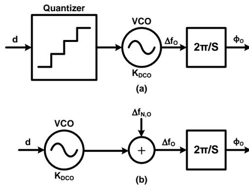
Fig. 3. 9 DCO quantization noise model (a) Behavior model and (b) mathematic model
