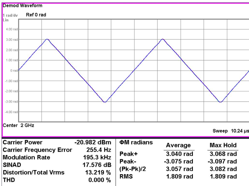
Fig. 7. 12 Demodulated dual-slope ramp PM signal
