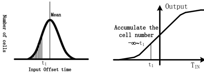
Fig. 3. 20 Time offset distribution and TDC input-output characteristic
