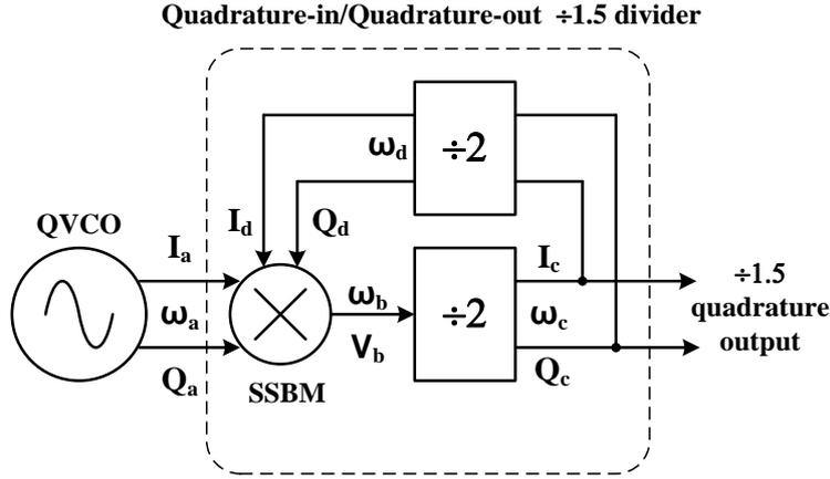
Fig. 4. 4 Block diagram of a Quadrature-in/Quadrature-out ÷1.5 divider
