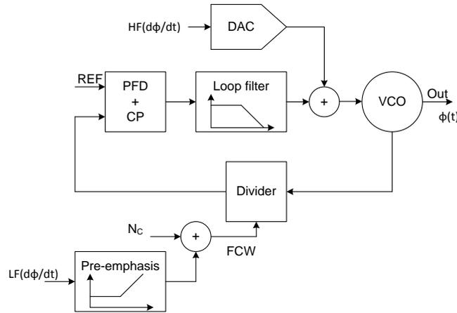
Fig. 5. 2 Block diagram of PLL based wide band PM
