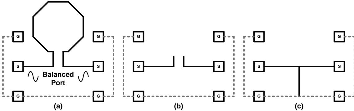
Fig. A-I.2 Testing structure for (a) inductor, (b) open de-embedding and (c) short de-embedding
