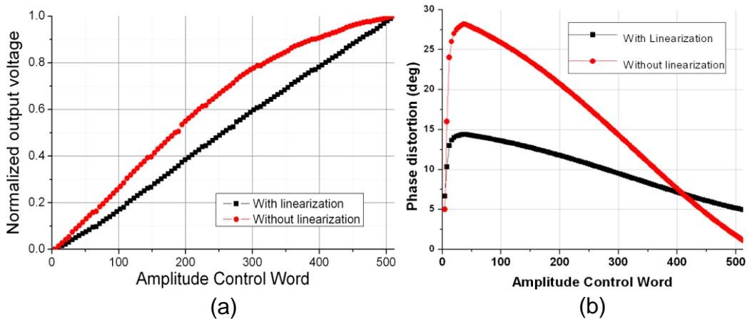
Fig. 6. 14 Measured static transfer characteristic with 2GHz output and 13.7dBm peak output power: (a) AM-AM and (b) AM-PM
