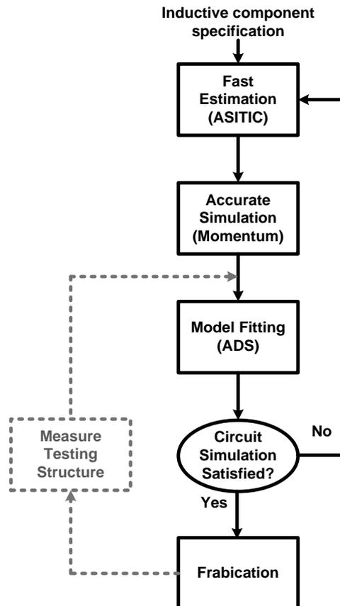
Fig. A-I. 1 Design flow of the inductive components
