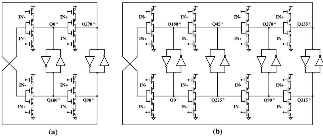
Fig. 4. 9 implementation of the divider (a)  $\div 2$ , 4-phases and (b)  $\div 4$  8-phases output
