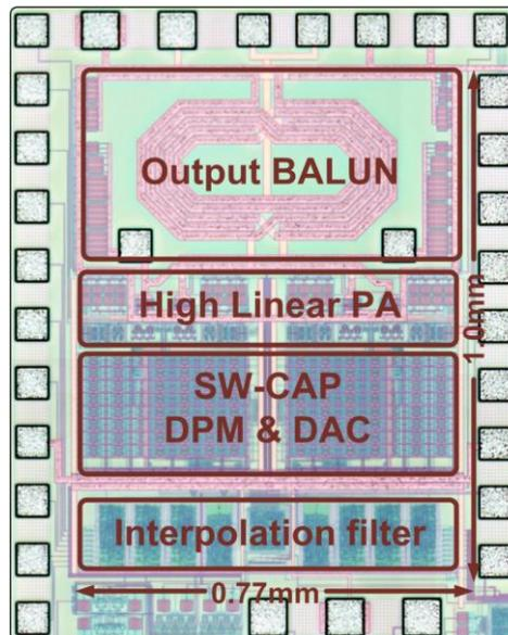
Fig. 6. 17 Die micrograph of the proposed transmitter
