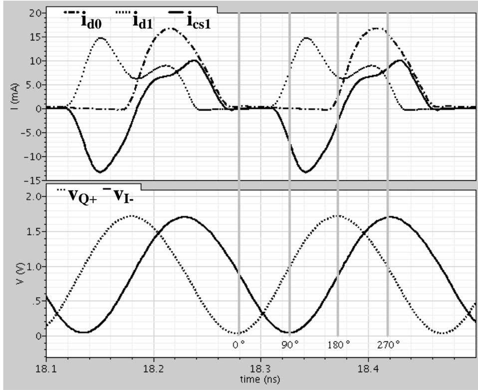
Fig. 3. 7 Transient current and voltage waveforms of M0 and M1
