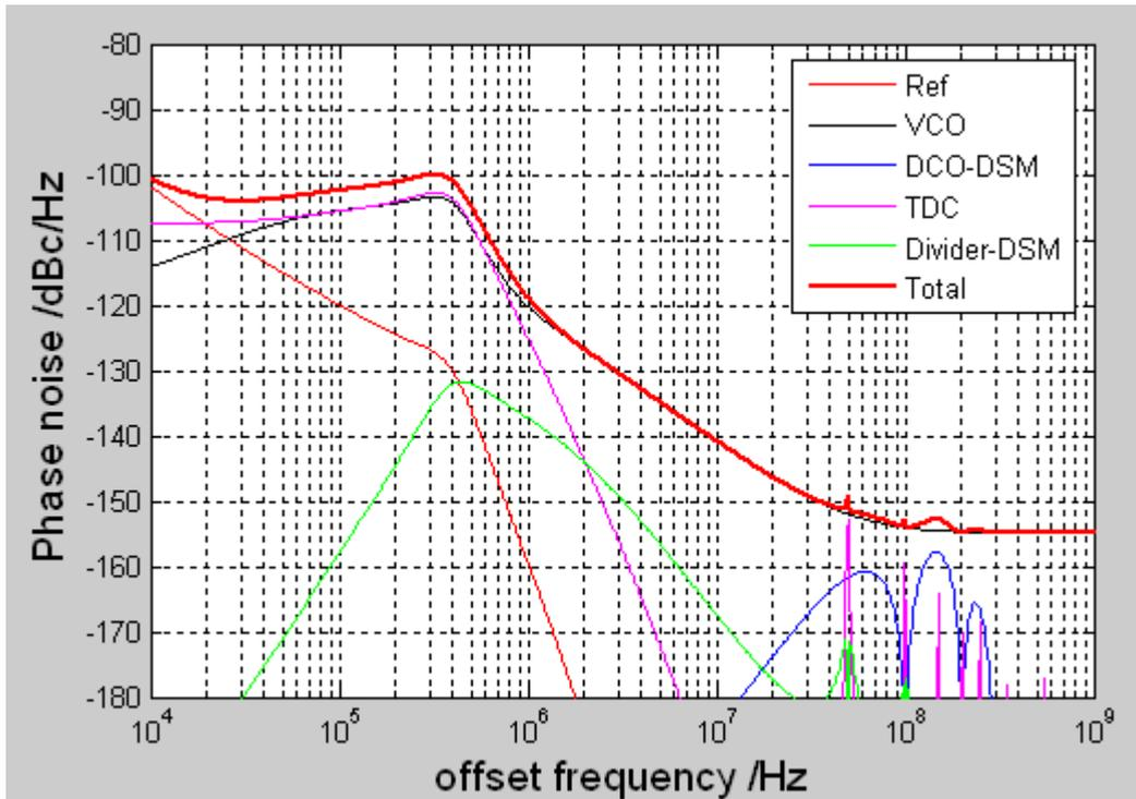
Fig. 3. 36 Phase noise simulation of the ADPLL
