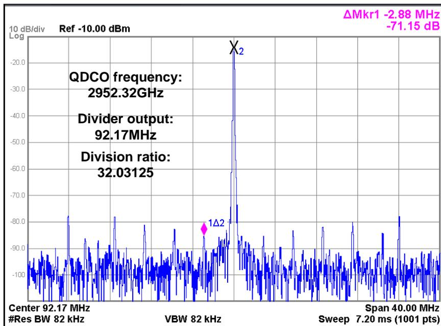
Fig. 7. 7 Worst case output spurs of the sub-integer programmable divider
