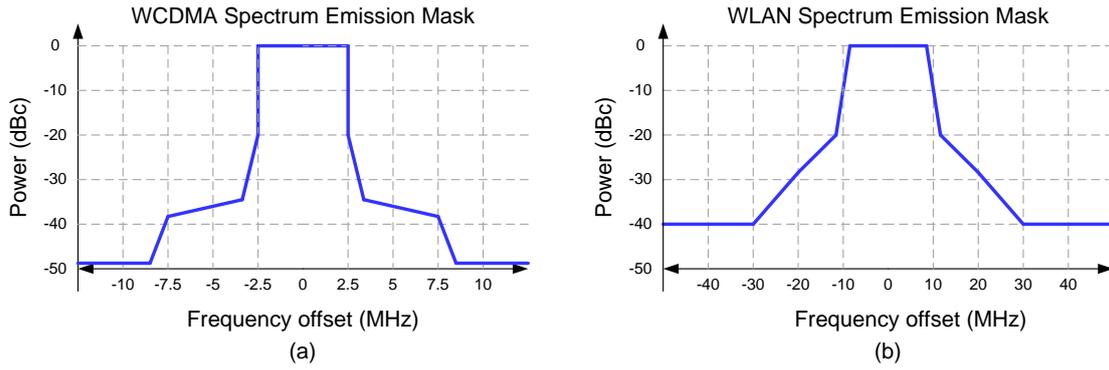
Fig. 2. 7 Spectral mask (a) WCDMA (b) WLAN 802.11 b/g
