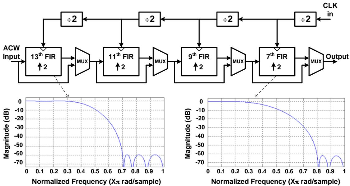
Fig. 6. 12 Block diagram of the proposed digital interpolation filter
