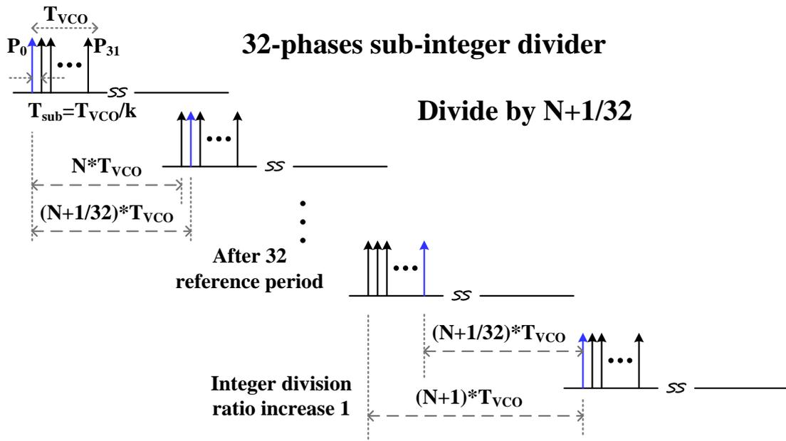
Fig. 3. 29 Operation principle of the Phase-interpolated programmable divider
