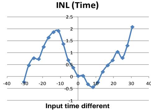
Fig. 3. 24 Measured INL error with TDC gain = 4
