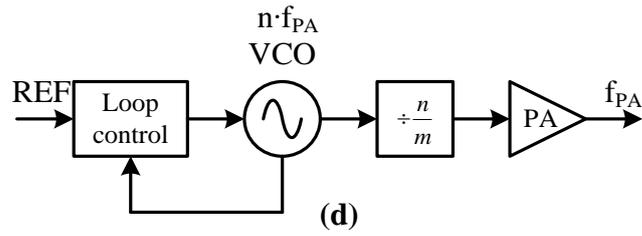
Fig. 4. 2 Pulling reduction techniques for LO generation: (a) Integer frequency division, (b) tunable delay for in/out phase pulling, (c) phase diagram of in/out phase pulling, and (d) fractional frequency division
