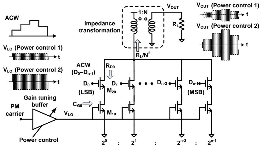
Fig. 6. 3 Illustration of the operation of the switched-current DPM
