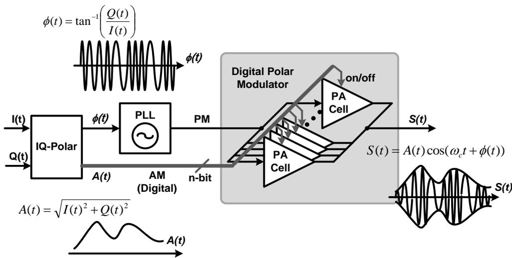
Fig. 6. 1 Block diagram of a typical digital polar modulator architecture
