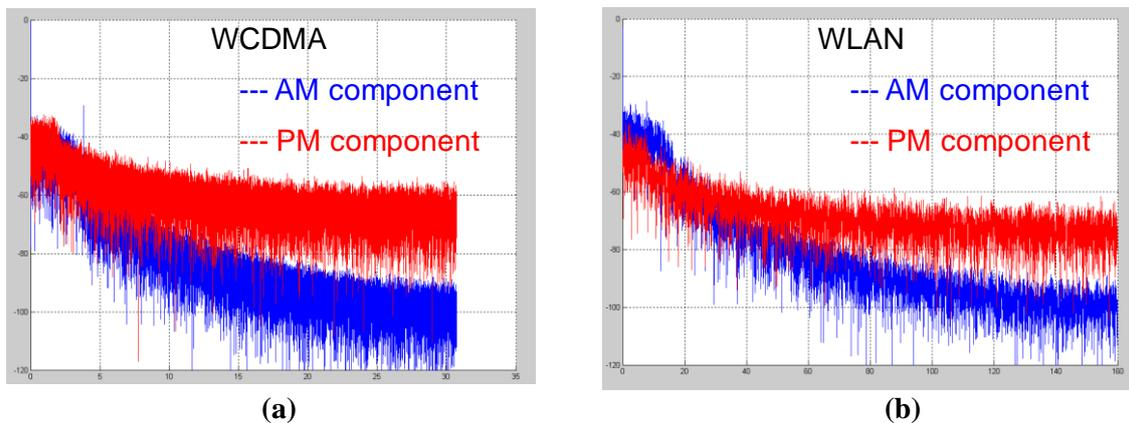
Fig. 2. 13 Frequency spectrums of the AM and PM components for WCDMA and 20MHz WLAN
