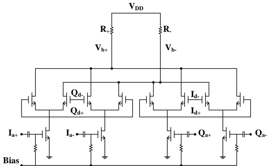
Fig. 4. 5 a classical circuit implementation of the SSBM
