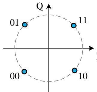
Fig. 2. 3 constellation diagram example for QPSK
