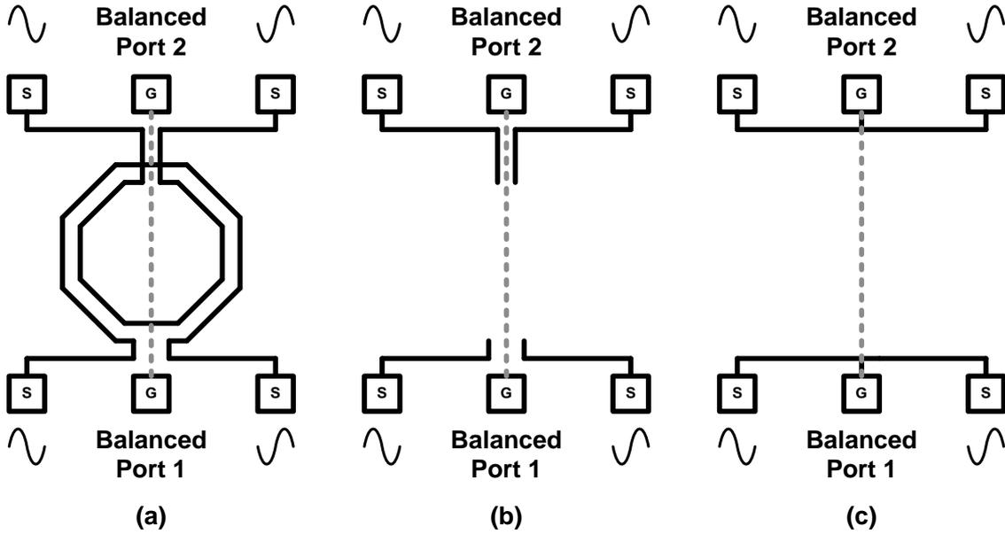
Fig. A-I.3 Testing structure for (a) Transformer, (b) open de-embedding and (c) short de-embedding
