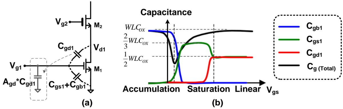
Fig. 6. 9 Common-source cascode PA: (a) schematic showing input capacitances, and (b) the input gate capacitance versus  $V_{gs}$
