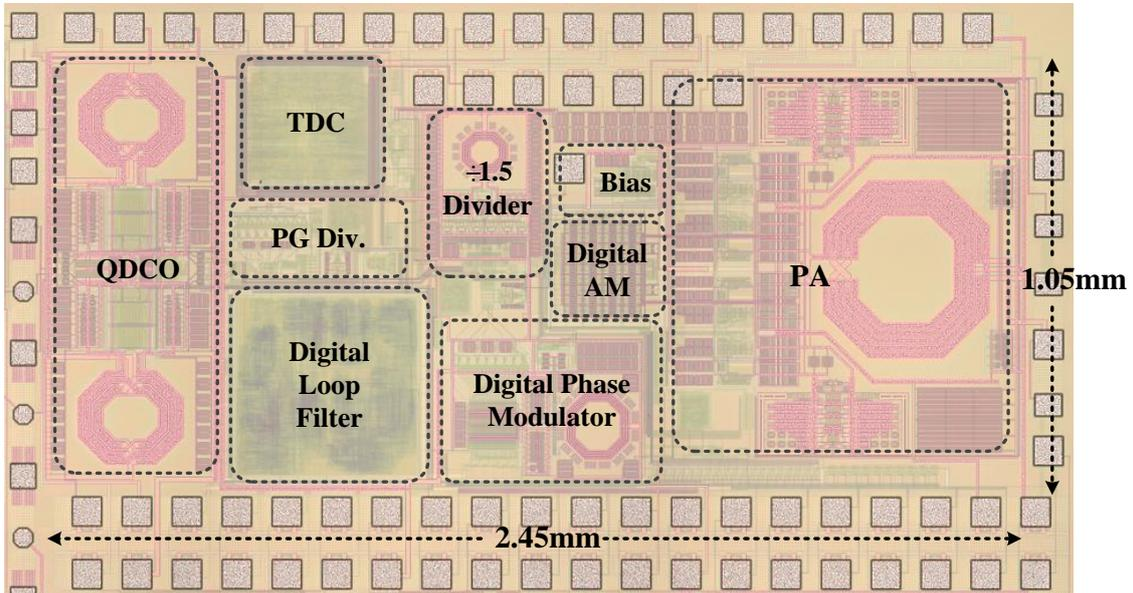
Fig. 7. 2 layout of the transmitter system
