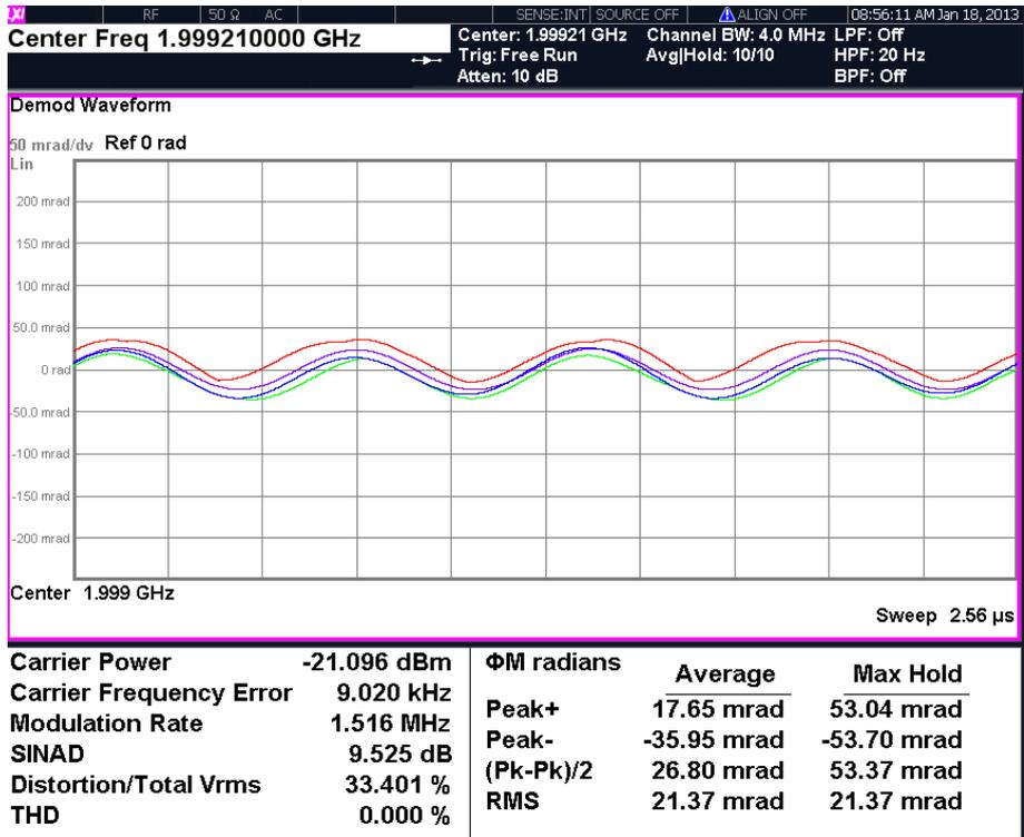
Fig. 7. 14 PM phase error measurement
