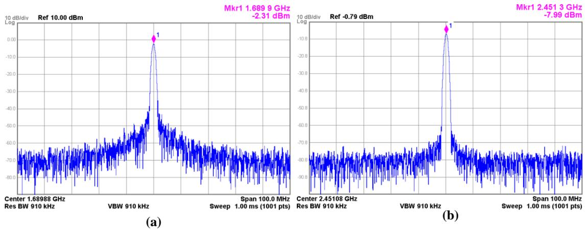
Fig. 7. 10 Measured output frequency range of the  $\pm 1.5$  divider (a) minimum frequency and (b) maximum frequency
