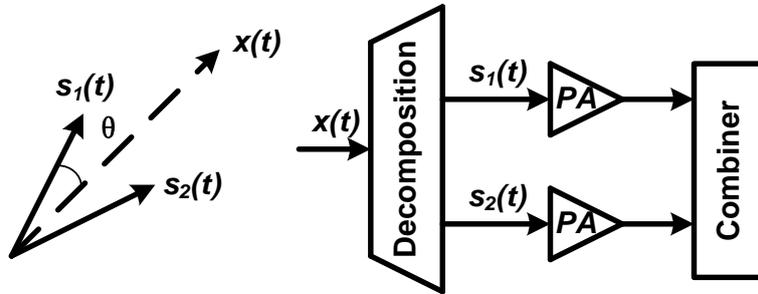
Fig. 2. 10 Block diagram of the outphasing transmitter
