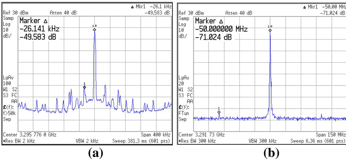
Fig. 7. 9 Measured ADPLL spurs (a) in-band fractional spurs and (b) reference spurs
