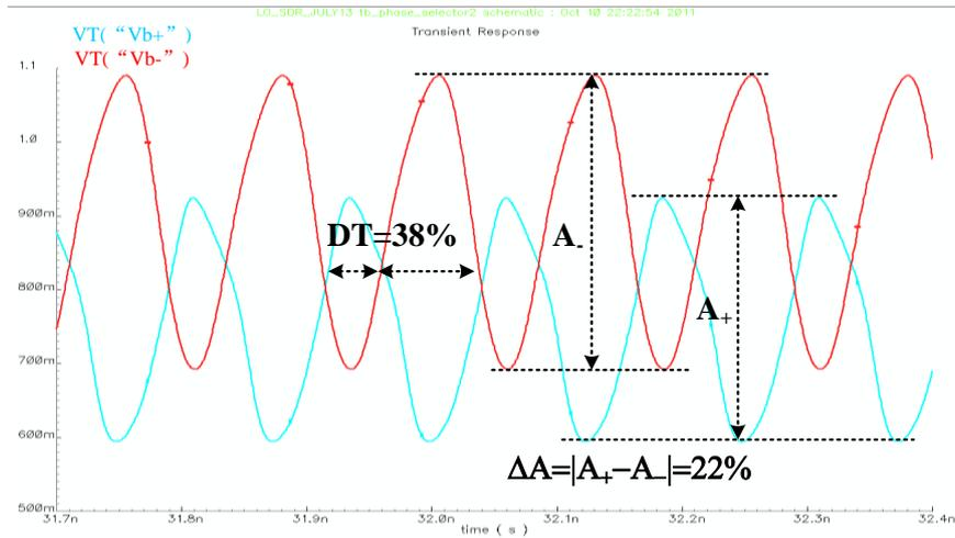
Fig. 4. 6 simulated SSBM output
