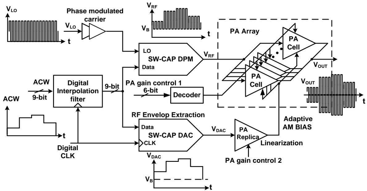
Fig. 6. 4 Block diagram of the proposed digital polar transmitter
