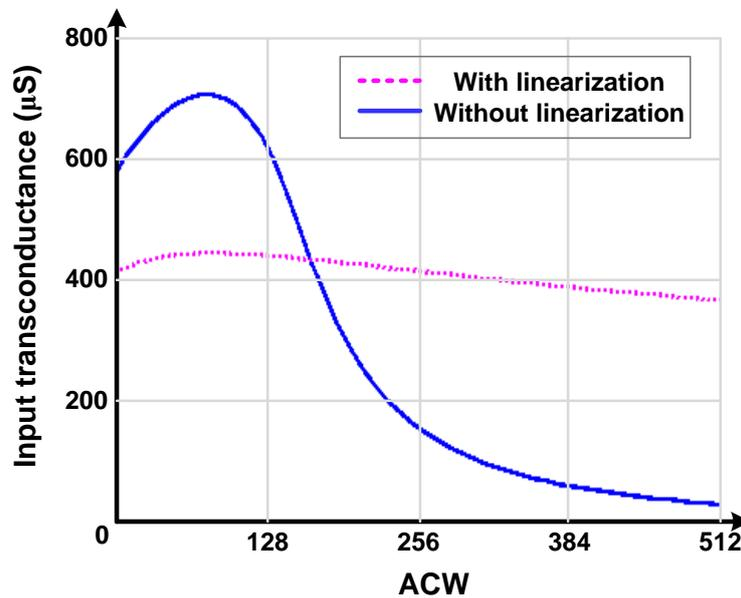
Fig. 6. 10 Simulated PA input transconductance versus ACW
